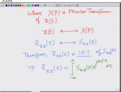
Now look at this we have  $S \times x F$  equals Fourier transform that is if we look at  $R \times x$  tao that has Fourier transform  $S \times x$  of F therefore S or  $SR \times x$  of tao is the inverse Fourier transform is IFT is the IFT of  $S \times x$  of F, alright. This is the inverse Fourier transform S which implies  $R \times x$  of tao can be expressed as integral - infinity to infinity  $S \times x$  of F e power F power F and F tao d tao, correct?
