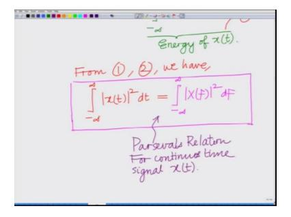
And from here we have R x x zero is basically integral - infinity to infinity magnitude X(F) square d F. So from this result let us call this result as 1 and let us call this result as 2. From 1, 2 we have that is R x x zero from results 1, 2 we have integral - infinity to infinity magnitude x(t) square dt equals integral - infinity to infinity magnitude X(F) square dF. And this is nothing but this is the Persavals relation.
