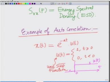
Let us consider this function or let us consider this signal x(t) equals to e power - at u(t) where u(t) as we are all familiar is the unit step function which is 1 for t greater than equal to zero, for t less than equal to zero this is known as the unit step. This is known as the unit step function, correct, this is zero for t less than equal to zero, correct? And for t greater than or equal to zero this is one.
