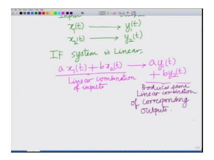
So what I would like to do is look at the transmission of a signal through a linear system, alright. So what we have is basically, let us consider a signal that is considered signal x(t) given as an input to a LTI where LTI denotes basically a linear time invariant system. This system this system has is very relevant and very important as for signal processing and communication, alright. So let me just briefly describe what is an LTI system?
