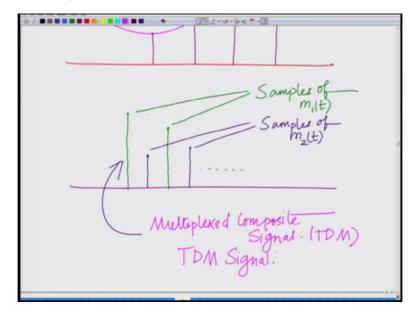
So what we are going to have over here are basically if you look at this what we are going to have is we are going to have a sample of m1(t) correct we are going to have the first sample of m1(t) followed by the sample of m2(t) correct. So this will be followed by the sample of m2(t) then we will have another sample of we will have another sample of well m1(t) followed by another sample of m2(t) and this will proceed so on and so forth.
