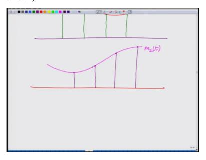
And let us say we have another signal m2(t) now remember the sampling instance of m2(t) have to between be between those of m1(t) because we have a commutator which is sampling let us say m1(t) followed by m2(t) and alternately repeating this procedure so we have the samples of m2(t), these are the samples of m2(t).
