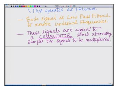
So these signals are subsequently applied to a to a commutator ok this is a special device commutator which alternately samples the signals to be multiplexed. So these are applied to a commutator which alternately samples the signals to be multiplexed, ok.
