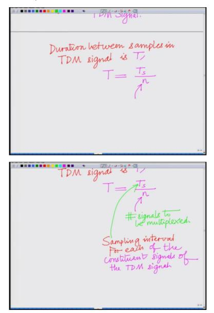
So duration between samples is T where T equals TS by n, so this is the duration between samples n we have noted is the number of signals to be multiplexed and TS is the sampling duration TS is the sampling interval TS is the sampling interval for each let us right this sampling interval for each individual signal or each of the constituent signals in the TDM signal each of the each of the constituent signals of the TDM signal, ok.
