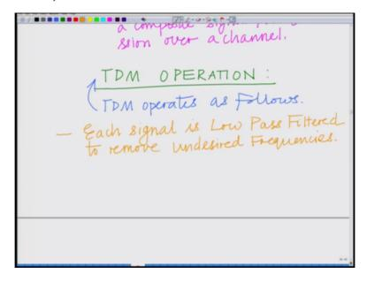
And now so TDM so let us look at operation of TDM let us look at the operation of TDM, TDM operates as follows each signal so TDM operates as follows each signal is first low pass filtered to remove undesired. So in the first step each signal each signal is low pass filtered to first remove the to remove the undesired frequencies, ok.
