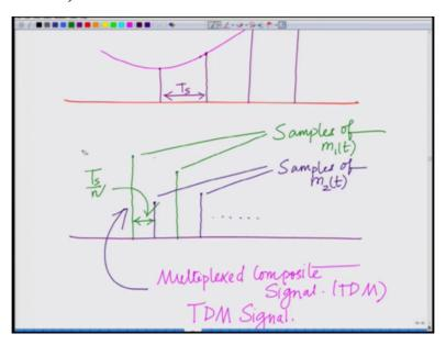
Then in TS if N signals are sampled well you have N samples for each TS duration therefore the duration between these samples of the composite signal is well TS divided by N, in this case it is TS divided by 2.
