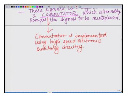
And this commutator is implemented this commutator this commutator is implemented using high speed electronic switching circuitry using high speed is implemented using high speed electronic switching circuitry.
