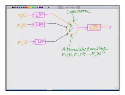
So if I look at a schematic of this diagram the schematic looks as follows. So I have m1(t) that is the first signal similar to your Frequency Division Multiplexing I have m1(t), ok which is the first signal to be multiplexed, m2(t) so on upto mn(t) these are the N signals to be multiplexed, ok.
