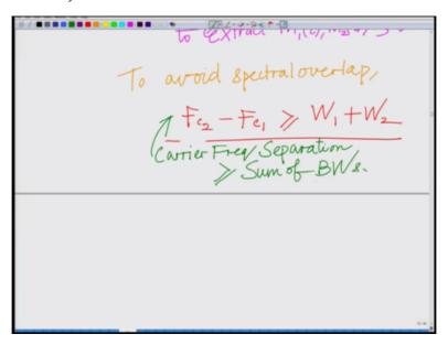
To avoid overlap to avoid overlap we must have Fc2 minus Fc1 greater than or equal to W1 plus W2, ok. This means that basically your carrier frequency separation must be greater than separation must be greater than or equal to the sum carrier frequency separation must be greater than or equal to sum of bandwidths now this is for DSB, ok.
