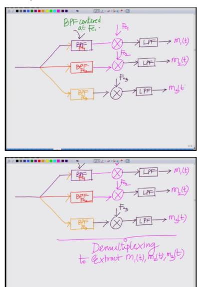
Next we have Bandpass filter centered at Fc2 demodulate with carrier frequency Fc2, Bandpass filter centered at Fc3 demodulate with carrier frequency Fc3, ok. And then we are able to separate, ok so this will give us your m1(t), give you your m2(t), this will give you m3(t). Now this is basically a Demultiplexing Demultiplexing to extract m1(t), m2(t) and m3(t), ok demultiplexing is nothing but you have a composite signal from that you are extracting the separate component m1(t), m2(t), m3(t).
