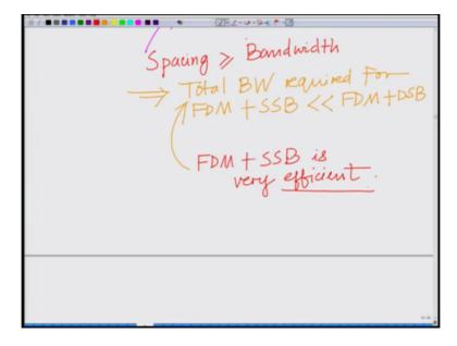
Therefore FDM plus SSB is much more efficient and comparison to FDM Frequency Division Multiplexing with DSB Double Sideband, so FDM plus SSB so which implies FDM plus SSB is very efficient FDM plus SSB is very efficient.
