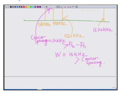
However the message bandwidth W is typically around 15 kilohertz alright so W is approximately equal to which is basically greater than your carrier spacing, which means that
