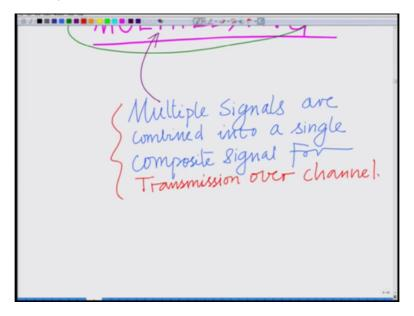
So the key idea behind multiplexing is that multiple signals multiple signals correct multiple signals are combined multiple signals are combined into a single composite for transmission over the channel transmission over the channel ok so multiple signals are combined into a single what is the advantage of this the advantage of this is you are using the same channel right the same channel for the transmission of multiple signals instead of a single signal ok.
