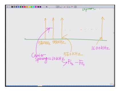
Now carriers spacing is 10 kilohertz, the carriers are spaced 10 kilohertz apart. So carriers are spaced 10 kilohertz apart, so if you look at carriers these are spaced so you start at 540, 550 kilohertz than you have the next carrier at 560 kilohertz so on and so forth you will have carrier the last carrier will be at obviously this is not according to scale the last carrier will be at 1600 kilohertz.
