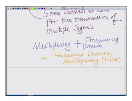
So this makes the channel usage efficient so channel so same channel is used for the transmission of multiple signals. So basically the channel usage becomes very efficient, ok. And now multiplexing is done in the frequency domain so there are various ways to do multiplexing so when multiplexing is done in the frequency domain that becomes Frequency Division Multiplexing, ok.
