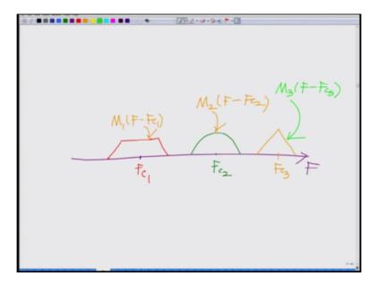
So the spectrum of the combined signal will now look as follows the composite signal spectrum, if you look at the spectrum of the composite signal the spectrum of the composite signal will look as follows, I will have in the frequency domain this is F, I will have the spectrum 1 that is translated to I will have spectrum 1 that is translated to that is translated to Fc1, ok. This is your spectrum 1 which is translated to Fc1, correct.
