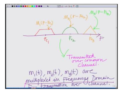
For instance to extract M1 I have to filter at Fc1, if I have to extract M2 I have to consider Bandpass filter centered at Fc2, to extract M3 I have to consider Bandpass filter centered at Fc3.
