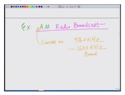
Let us take a simple example example of AM broadcast again or AM Radio Broadcast AM is amplitude modulation AM Radio Broadcast. In AM Radio Broadcast we have carriers in the 540 kilohertz to 1600 kilohertz band, ok.
