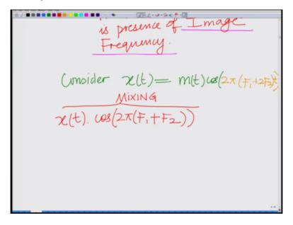
Now what is an image frequency, now consider the signal incoming signal x(t) equals m(t) cosine(2pi(F1 plus 2F2 F1 plus 2F2)t), ok F1 plus 2F2(t), ok. Now this is mixed with again cosine 2pi F1 again this is mixed heterodyne with cosine 2pi F, so we perform x(t) into cosine 2pi(F1 plus 2F2). So this is signal this is mixing, ok so this is mixed with a signal with frequency F1 plus F2.
