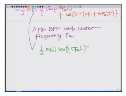
Now if we band pass filter this if we band pass filter this signal the band pass filter at F2 of suitable band width what you can see is we can extract the cosine 2pi F2t component ok. So now after band pass filtering with center frequency after band pass filtering with center frequency F2 what we obtain after BPF what we obtain is half m(t) cosine (2piF2t), ok.
