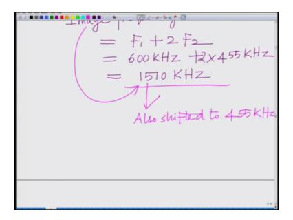
Now the image frequency corresponding to this the image frequency that is F1 plus 2F2 that is equal to 600 kilohertz well plus twice into (450) 2F2 twice into 455 kilohertz ok so that will be your 1510 kilohertz so this is the image frequency (1510) this is also shifted to so incoming signal with this also shifted to to 455 kilohertz, ok.
