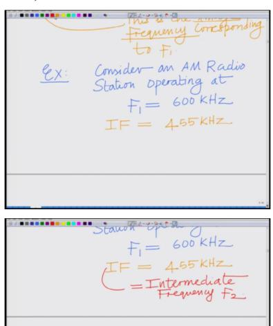
For example let us take an example ok consider an FM station or consider an AM station AM Radio Station operating at operating at F1 equals let us say this is operating at F1 equal to 600 kilohertz. We choose an intermediate frequency IF equals when intermediate frequency ok, remember IF stands for intermediate frequency, so intermediate frequency that is your F2, ok.
