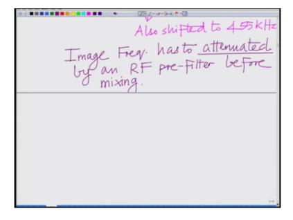
So this has to be removed so to avoid interference so image has to be image frequency signal image frequency has to be suitably attenuated by an RF by an RF pre-filter before by an RF pre-filter before mixing ok so image filter has to be attenuated by an RF filter otherwise it is going to interfere with that desired signal which is being translated to the intermediate frequency, ok alright so that is the problem with the image frequency.
