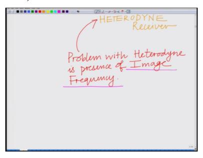
And the problem with the heterodyne receiver is the presence of what is known as an image frequency so problem with heterodyne is the presence of is the presence of what is known as an image what is known as an image frequency.
