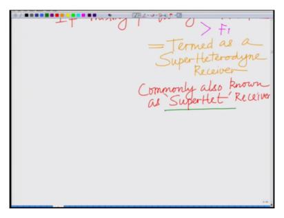
Now if mixing frequency the more popular version if mixing if the mixing frequency equals F1 plus F2 which is greater than which is greater than F1 this is termed as a super heterodyne this is termed as a or commonly also known as a super het simply known as a super het receiver this is commonly also known as a super het receiver, ok this is also commonly simply known as the super het receiver.
