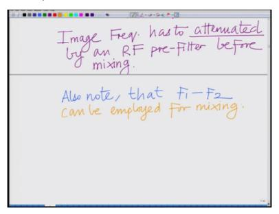
Realize that in the heterodyning also note that we have used F1 plus F2 with the heterodyne that is as the frequency of the locally locally generated oscillator (freq) frequency of the locally generated carrier wave ok. Now realize that one can also use F1 minus F2 where F F2 is the intermediate frequency so also note also note that F1 minus F2 F1 minus F2 can be employed for mixing.
