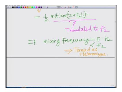
And now again once again if we band pass filter at F2 employing no if you band pass filter band pass filter at center frequency F2 this will yield half m(t) cosine (2piF2t), that is basically employing F1 that is mixing with F1 minus F2 also one can translate to the one can translate signal incoming signal with carrier frequency F1 to the intermediate frequency F2, note that this is also translated also translated to F2, ok.
