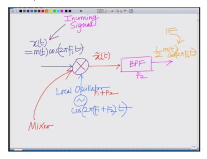
And therefore the output of this will be half m(t) cosine (2piF2t). This is your IF signal intermediate frequency signal, ok.
