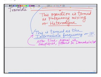
After this the signal is amplified, filtered and demodulated after this amplified, filtered and after this the filter is after this the signal is amplified, filtered and demodulated, ok. So this is termed as the intermediate so all the frequencies the modulated signals are translated for common center frequency and new center frequency which is termed as the intermediate
