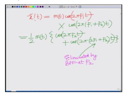
Now let us examine this output x tilde (t) x tilde (t) equals this is equal to m(t) cosine (2pi F1t) times that is your x(t) times cosine (2pi(F1 plus F2)t) that is a career frequency of the mixer that gives me half m(t) {cosine (2pi F1t) into cosine (2pi(F1 plus F2) into F2 t) so this is half cosine 2pi F1 plus F2 minus F1 F2 t plus cosine (2pi F1 plus F1 plus F2 that is 2F1 that is basically you are your (2F1 plus F2) t)}.
