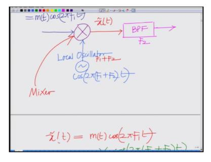
Therefore what we have to do is at the output we have to pass it through a band pass filter centered at F2.
