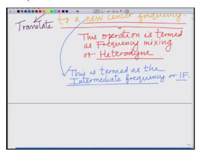
And this new center frequency alright this new center frequency is common center frequency to which all the received centers signals are translated this is termed as the intermediate frequency IF this new center frequency this is termed as the intermediate frequency or IF, ok.
