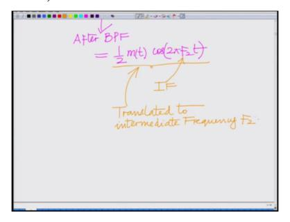
So now you can see it is translated to this new frequency F2 where F2 is the intermediate frequency so this F2 is nothing but IF that is the intermediate frequency. So this is translated translated to the intermediate frequency F2 translated to the intermediate frequency F2.
