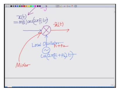
So you are mixing it with the different frequency that is the whole idea so I am demodulating this with a different frequency I am mixing this, so this is a local oscillator. Now in a coherent demodulator we demodulate with the same frequency F1 is the frequency career frequency of the incoming signal we demodulate it with F1 but here we are using we use a different frequency F2 alright demodulating or mixing with this frequency multiplying with this frequency career of frequency F2, ok.
