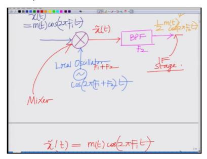
So basically what we are doing is we have this F1 incoming signal with incoming signal with carrier frequency F1 mixing with we are mixing with locally generated carrier which has frequency F1 plus F2 and therefore after you band pass filter the output you get the next signal with at the intermediate frequency m(t) half m(t) cosine (2piF2t) which is at the intermediate frequency IF F2. So this is the IF stage. So basically this is your intermediate frequency stage.
