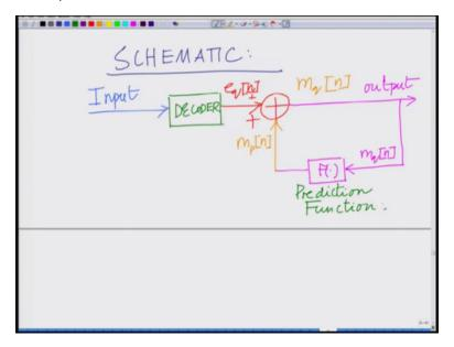
So let us draw a schematic for the reconstruction the schematic for the reconstruction will be very simple you have your input, okay from the channel or your storage device which is the encoded input you pass it through a decoder remember this is an encoded bit stream you pass it through the decoder, alright eq[n] is encoded to produce the bit stream encoded bit stream is passed through the decoder that gives us again eq[n] that is the quantized error to eq[n] you add mp[n].
