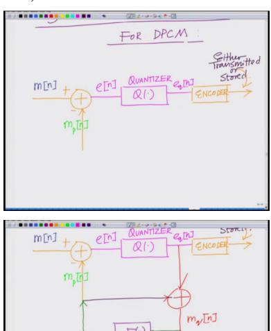
Now we can now a schematic diagram for this (())(17:39) for DPCM, okay this is a schematic diagram for differential pulse coded modulation, now we have your signal sample m[n] similar to delta modulation we take in the sample at every time instant n, okay now from this we subtract the prediction this is minus m[n] that is the prediction, okay we subtract the prediction m[n], okay that gives us e[n] which is quantized this is your quantizer to get the quantized error eq[n].
