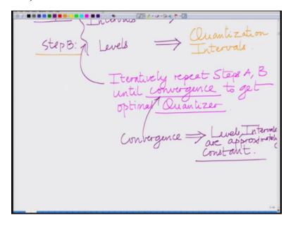
So the algorithm will be iteratively okay iteratively repeats step until convergence okay until non the levels and the intervals and the levels are not changing basically that is what it means until convergence to get the optimal quantizer.
