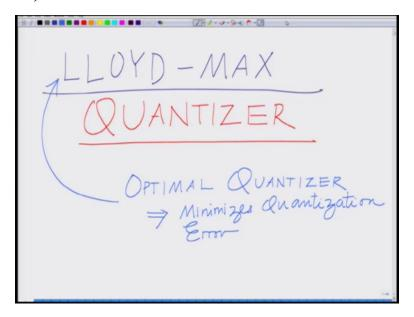
So you want to look at the Lloyd max the Lloyd max quantizer which is really a scheme to design the optimal quantizer. So the Lloyd max quantizer gives what is known as the optimal quantizer optimal meaning, it minimizes the error quantization error.
