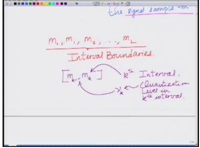
So to start with the Lloyd max quantizer we have to first consider we have to consider Fm(m) or let us make it symmetric this is your Fm(m) which is the this is your probability density function this is the we have to start with the Probability Density Function (PDF) of the PDF of the signal sample m, okay.
