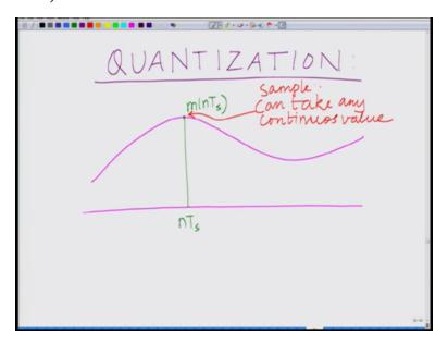
Now what is quantization remember we already know something that is we are sampling signals a discrete time instants, correct? So we have the signal and which we are sampling at the sampling instants the multiples of the sampling instants that this is the sample at mnTs at the nth multiple of the sampling.
