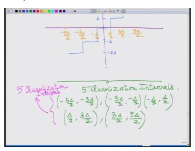
We have well, 5 quantization intervals the 5 quantization intervals are minus 5 delta by 2 to minus 3 delta by 2 minus 3 delta by 2 to minus Delta by 2 minus delta by 2 to delta by 2, delta by 2 to 3 delta by 2, 3 delta by 2 to 5 delta by 2, okay. So these are your 5 quantization intervals, okay. These are 5 quantization intervals and we are calling this as a uniformly spaced uniform quantizer because note that the widths of this quantization interval are uniform.
