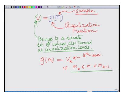
And therefore this process of quantization can be represented as follows now we have the sample m so m is the sample we have the quantization function gm so this maps it to nu, so this is the sample which can take any particular value so this is your sample this is your quantization function this is your quantization function and this bears the quantized this V belongs to a quantized station set.
