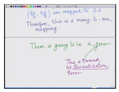
Therefore this is a first of all this is a many to one mapping there is a first point, second there is going to be a quantization error by definition there is going to be a there is going to be an error this is this is a many to one therefore it is a non-invertible mapping this is termed as quantization error this is termed as quantization error for instance, correct?
