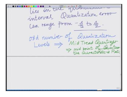
So odd number of quantization levels odd number of remember we have 5 quantization levels odd number of quantization levels implies we have a mid thread (quanti) which implies implies midpoint of quantizer the characteristic is flat that is midpoint not midpoint of quantizer basically the midpoint of the dynamic range that is if you will get the dynamic range minus 5 delta by 2 to delta by 2 5 Delta by 2 at the midpoint at the middle of the quantizer the quantization characteristic, right?
