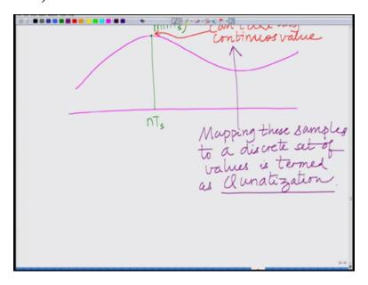
So converting this continuous valued samples conversion of these continuous (())(2:14) to a discrete or mapping these samples to a discrete set of values is termed as is termed as this is termed as quantization, okay. Converting samples this continuous samples which have continuous values to a discrete set of values or a discrete set of levels is termed as this process is termed as quantization, okay.
