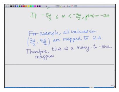
So this quantization error for example all values in all values in 3delta by 2 to 5 delta by 2 are mapped are mapped to 2 Delta therefore there is going to be a quantization error.
