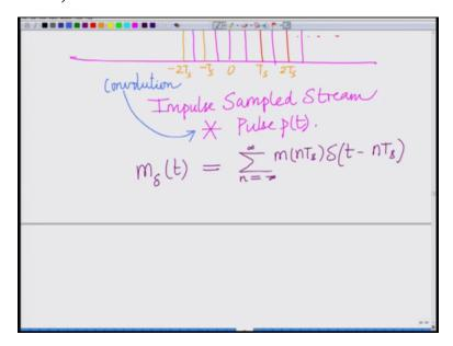
So our impulse sampled stream or impulse sampled signal is remember, m delta T equals well, summation n equal to minus infinity to infinity m of nTs into delta t minus nTs, okay. Now this is basically the convolution operator this star represents convolution, now I take this m delta t, correct?
