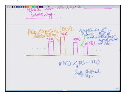
What we are also doing is we are modulating the amplitude of each pulse remember, we have a pulse at each nTs that is scaled by the value of the signal at nTs that is mnts times the pulse that is each pulse is of unit amplitude let us say and it is scaled by m nTs that is the value of the
