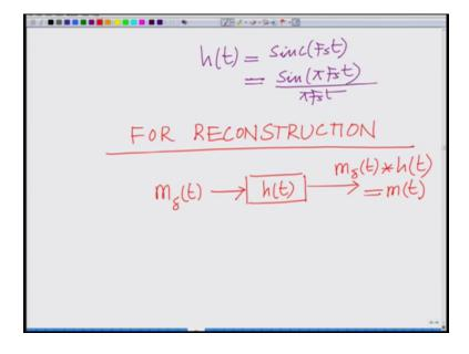
Now let us highlight that procedure for reconstruction we take our sampled signal m delta t pass it through the system with impulse response ht and that gives this, so m delta t convolved with h of t that gives back our original signal m(t) when there is no aliasing, right? Because we are a low pass filtering to extract the component at 0 frequency that is the component between minus Fm and Fm which is simply a replica of the spectrum of the original (sa) signal m(t) scaled by Fs.
