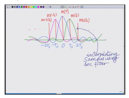
So what we are doing is literally, basically we are interpolating using the sinc filter this process is basically we are interpolating the samples. We are interpolating the samples using the sinc filter and what is our reconstruction?
