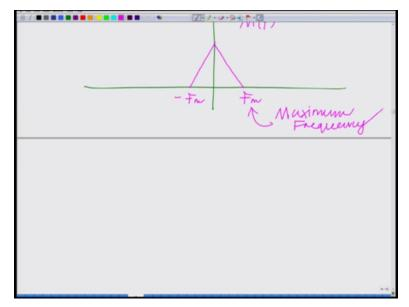
If you have your original spectrum that is MF which is has maximum frequency Fm let us say minimum frequency that is from minus Fm to Fm that is its support or where it is nonzero is from minus Fm to Fm the maximum frequency is Fm, this is the maximum frequency and therefore now what you are doing is basically you have Fs times MF.
