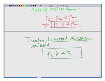
So aliasing occurs when occurs if Fs minus Fm is less than Fm that implies Fs less than 2Fm that is sampling frequency is less than twice the maximum frequency, so this is the condition for aliasing therefore to avoid aliasing we need we need Fs greater than or equal to 2Fm that is the minimum sampling frequency to avoid aliasing or the distortion caused by aliasing is Fs greater than equal to, to avoid aliasing we need Fs greater than equal to 2 Fm where Fm is the maximum frequency.
