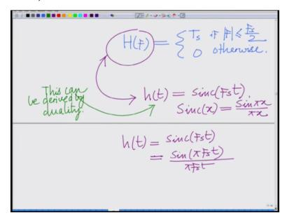
So this is the sinc function in the time domain and we can derive this and this can be derived by let us note that this can be derived by duality. And this can be derived by duality, okay. So this can be derived using this can be derived using duality, okay. And therefore what we have this can be derived by using the principle of duality we know that the principle of duality, okay. Now therefore we have the signal m(t), so what we have to do to reconstruct the signal for reconstruction.
