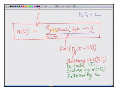
So what we are doing is basically we are shifting, correct? we are shifting of course there is no Fs there is no Fs because this is simply your mnts into Delta t minus Ts, so this is simply m of nTs so anyway what we are doing is basically we are taking each sinc Fs shifting it to nTs where as shifting sinc of Fst to each nTs to each nTs scaling by m mnts followed by the.
