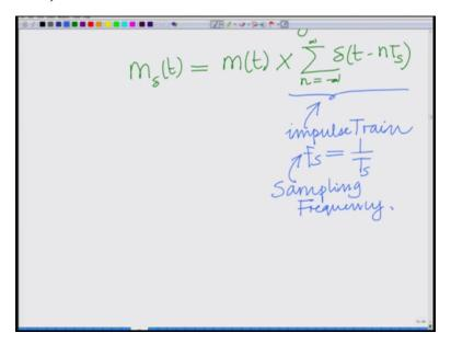
So this is your impulse train which is a series of impulses at every multiple of the sampling time interval Ts, okay where a sampling frequency Fs equals 1 over Ts, okay. Fs is the sampling frequency this is our sampling frequency and now we are multiplying m(t) by this (impul) (tra) impulse train that is m(t) times summation n equal to minus infinity to infinity delta t minus nTs and that each impulse at nTs, right? Picks the value of the original signal m at nTs.
