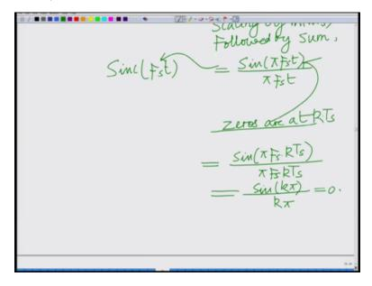
So what we have essentially is basically and remember sinc of Fnts sinc of Fst the zeros this is equal to basically (())(28:33) sin of pi Fst divided by pi Fst. So this is zeros are at the zeros of
