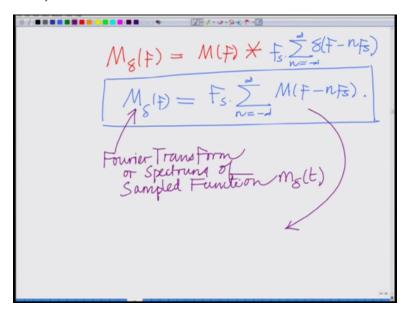
We said that m delta F is basically M of F convolved with since in the time domain we are multiplying in the frequency domain we have to convolved with the frequency response of the impulse train in the frequency for your transfer of the impulse train we have already seen is summation is Fs summation n equal to minus infinity to infinity delta F minus nFs which is equal to Fs summation n equal to minus infinity to infinity M of F minus Fs.
