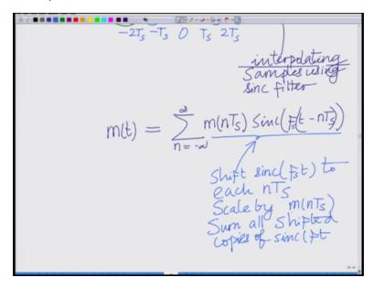
If you look at this relation over here that is m of t equals summation n equal to minus infinity to infinity m of nTs sinc of F Ts minus nTs that is this is basically shift that is basically shifts sinc FTs to each nTs scaled by mnTs and sum all shifted copies of this function sinc of sorry this is
