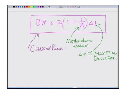
Now we combine these 2 principles so we combine combining these 2 principles Carson's rule (())(8:27) of FM signals the Carson's rule for bandwidth of FM signals is given as well the bandwidth of an FM signal is approximately equal to twice one plus one over beta into delta F where beta remember beta is the modulation index and Delta F equals the peak frequency deviation or peak or maximum frequency deviation, okay.
