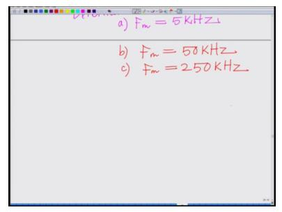
So let us look at a simple example for instance let us consider a carrier frequency equals 10 megahertz and Delta equals 50 kilohertz, now we would like to determine the bandwidth the bandwidth for FM corresponding to a) for FM that is values of Fm the maximum frequency FM
