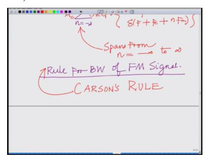
So what we would like to find is a rule, we would like to find the rule for a bandwidth of FM signal and this rule which gives us the bandwidth of an FM signal this is termed as the Carson's rule this is the Carson's rule, okay. So this is the rule which gives us the bandwidth, alright which helps us evaluate the bandwidth of the FM signal.
