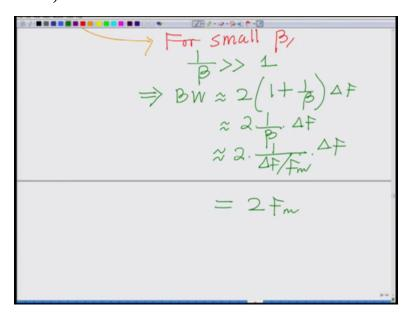
But remember beta is Delta F by FM so this is approximately twice 1 over Delta F by Fm into delta F which is equal to Fm which is equal to basically FM or let me just write this a little bit clearly. So this is 1 over delta F divided by FM into Delta F which is equal to twice which is equal to twice Fm, okay.
