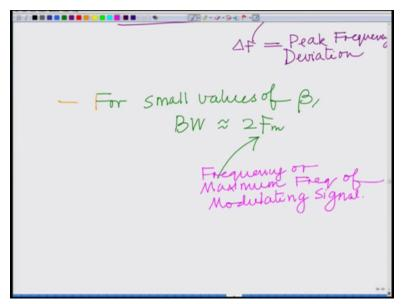
So for large values of data the bandwidth approaches Delta F however for small values of the modulation index beta for small values of for small values of beta the bandwidth is approximately 2Fm so 2Fm remember 2Fm is the frequency or you can think of it as a maximum frequency of modulating signal is either frequency or maximum frequency or the maximum frequency of maximum frequency of the modulating signal, okay.
