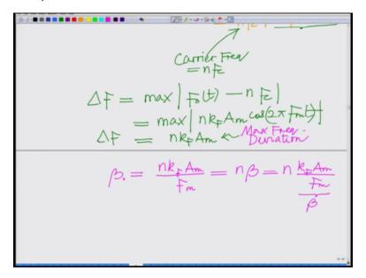
So carrier frequency is n times Fc delta F that is frequency deviation is Max your Fot minus n times Fc which is equal to max n times kF Am cosine two pi Fmt and this is equal to n times kF Am, so delta F the maximum frequency deviation, okay. So this is basically your maximum frequency deviation or peak frequency deviation.
