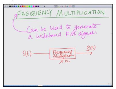
So what we can do to generate a wideband wideband frequency modulated signal I can use a frequency multiplication, okay. So frequency multiplication this can be used to generate can be used this can be used can be used to generate a wideband signal, okay. So what do we, so what do we mean by frequency we pass our narrowband FM signal through a frequency multiplier,
