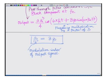
So the output beta so the modulation index beta output is the, this is the output modulation index or modulation index of the output signal. Modulation index of the modulation index of output signal is 3 times beta where beta is the modulation index of the input signal. Similarly we can consider other non-linear devices which are of the form raised to the which other forms signal raised to the power of n and that results in a frequency component output frequency component at nFc.
