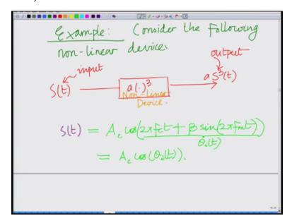
So consider so that is the key we would like to use a non-linear device for frequency (multi) for example, okay for example consider the following non-linear device consider the following non-linear device where our input is S(t) this is your non-linear device which performs a cube Law operation, so the output is a s cube of t, so input this is your input and this is your this is your output which is a times S cube t and you can clearly see this is a cubing operation.
