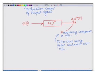
okay so if we consider to multiply it by a factor of n in general I can consider a non-linear device which is a raised to the power of n and therefore output will be a Sn to the power of t this will contain frequency component at nFc as we have seen raised to the power of 3 contains frequency component 3 Fc, in general signal raised to the power of n will contain frequency component at nFc.
