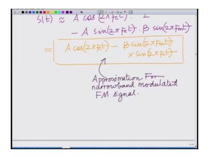
So substituting these we have Ac cosine two pi this is approximately equal to Ac cosine two pi Fct one minus A sin two pi F that is sin two pi Fct into beta sin two pi Fmt which is equal to A cosine two pi Fct minus beta cosine two pi Fmt into sin two pi Fct and this is the approximation for your narrow band modulated, so this is basically we are going to employ this approximation for the narrowband modulated FM signal.
