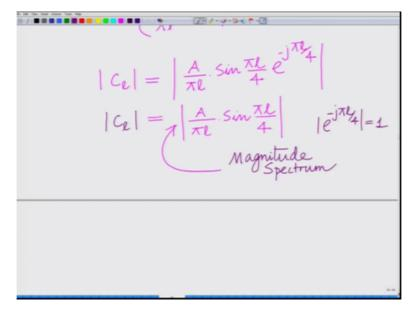
And further we can look at the magnitude, that is magnitude of this signal CL is magnitude Pi L sine Pi L by 4 e to the power of minus j Pi L by 4 and magnitude A to the power of minus j
