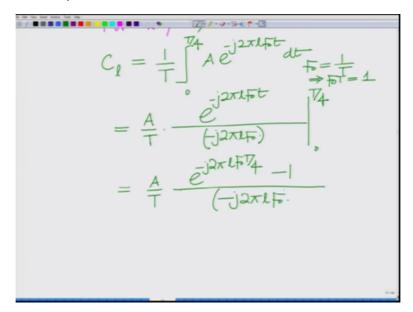
Now let us evaluate the rest of the cominusefficient the general CL for L not equals to 0 we have C L equals to 1 over T integral 0 to T by 4 A e to the power of minus j 2 Pi L F0 t dt, which is basically bringing A outside A over t integral e to the power of minus j L F0 t is e to the power of minus j 2 Pi L F0 t divided by minus j 2 Pi L F0 from the limits 0 to T by 4 and
