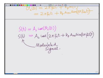
So this is your theta i t the net modulated message signal is given by st equals Ac cosine theta i t which is basically your Ac cosine 2pi Fct plus kP Am sin 2pi Fct this is the modulated signal, okay. St is your st is the modulated signal, okay. Now Fi(t) that is we have theta i t.
