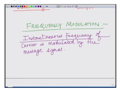
So frequency modulation is another kind of angle modulation so frequency modulation so let us now come to frequency modulation in the frequency modulation instantaneous frequency of the modulator scared so the instantaneous frequency of carrier is modulated by the message signal. So in this what we have is the instantaneous frequency is modular rather than the phase in the phase modulation the phase of the signal carrier is modulated by the message which results in phase discontinuity.
