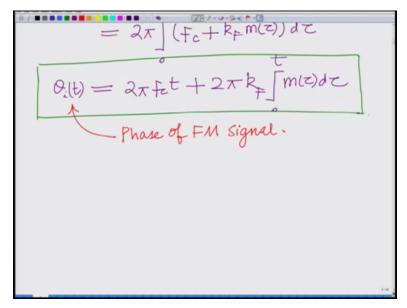
So therefore the phase now remember the phase frequency is the rate of change of phase therefore the phase of this is given as theta i t equals 2pi integral 0 to t Fi Tau d Tau which is basically 2pi integral 0 to t Fc plus kF m Tau d Tau which is equal to 2pi Fct plus 2pi integral 0 to t kF or rather 2pi kF since kF is a constant 0 to t m Tau t Tau that is your theta i that is your theta i this is the phase this is a phase of the frequency modulated signal.
