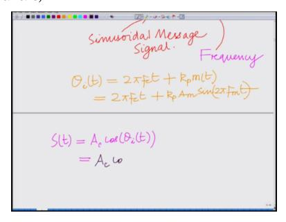
Therefore we have theta i t equals 2pi Fct plus kP times m(t) but we have m(t) is Am sin 2pi Fmt, so this is simply your 2 2pi Fct plus kP times Am sin 2pi Fmt.
