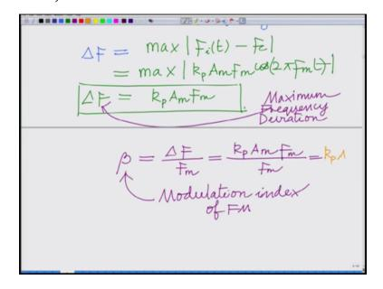
Now this is Fi(t) let us find the frequency deviation of this remember Delta F frequency deviation is the maximum of Fi(t) minus Fc there is a unmodulated frequency of the
