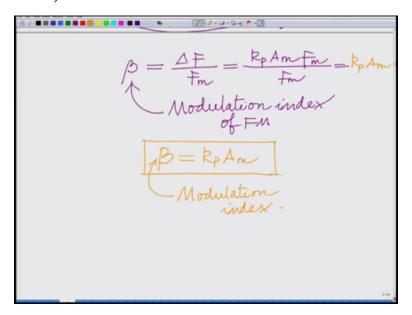
Therefore beta this is the modulation index equals kp times Am and look at this you can see this kp times Am this is also equal to the maximum phase deviation.
