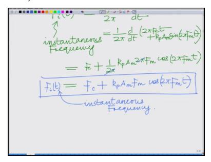
So this is kP Am Fm kP Am Fm into cosine 2pi Fmt this is the instantaneous frequency. This is your expression for the instantaneous frequency. This is the expression for the this Fi(t) this is the expression for the instantaneous frequency Fi(t) of this phase modulated signal phase which is modulated by the Sinusoidal message signal Am sin 2pi Fmt, okay.
