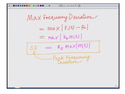
That is the expression for the instantaneous phase and further one can define the peak frequency deviation of this the maximum frequency deviation can be defined as well maximum you can see deviation can be defined as this can be defined as maximum of magnitude of Fi(t) minus Fc which is equal to the maximum of magnitude Fi(t) minus Fc you can see that is equal to kF times m(t) which is equal to well, kF times the maximum of magnitude m(t) that is your Delta F.
