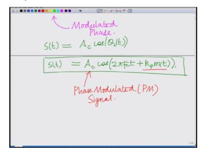
Now the modulated carrier is given as or the modulated signal is given as Ac cosine Theta theta it which is basically Ac cosine 2pi Fct plus kP times m(t) so this is a phase modulated signal. So this is your this is your phase modulated signal where the face of the signal is modulated by the message signal m(t), okay. And what you can see is because of this message signal where the phase is modulated by the message.
