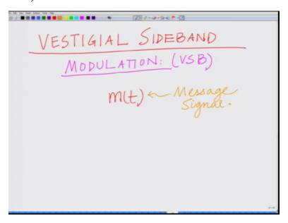
So the next topic or next different form of modulation that we are going to be interested in is vestigial sideband this is another form of modulation, we have seen single sideband modulation so this is vestigial sideband modulation also abbreviated as VSP vestigial sideband modulation. And we have already seen the motivation for vestigial sideband modulation and that can be expressed as follows, let me just remind you again why we need vestigial sideband modulation, okay.
