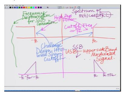
And the problem with this or rather the challenge is to generate high pass, the challenge of this to design high pass filter with such sharp such sharp cut-off frequency that is in fact practically very challenging if not impossible because frequently no matter how well your filter is designed it always has a small transition band, a transition band is a band in which it is transitioning from
