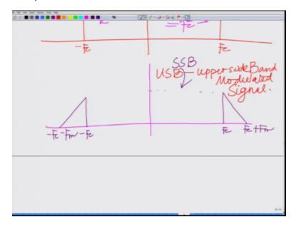
So this is Fc this is Fc plus Fm and again once again this is half m zero and similarly on minus Fc this is going to be minus Fc minus Fm and this is your SSB, correct? In fact this is your USB signal that is upper side band modulated signal this is the upper side band modulated signal and in fact to generate the lower side band modulated signal you have to pass it through an ideal low pass filter with cut-off Fc, okay.
