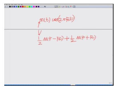
Now when we let us consider a modulated version of m(t) that is m(t) cosine two pi Fct which as we have well familiar has the spectrum half M(F) minus Fc plus half M(F) plus Fc that is M(F) shifted to Fc and M(F) shifted to minus Fc.
