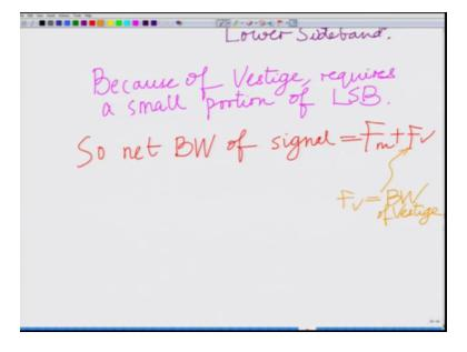
So this requires a bandwidth of because of the vestige you require because of the vestige that is small portion of the requires a small portion of LSB, so net bandwidth of the signal equals Fm plus Fv where Fv remember is the bandwidth of the Vestige. Fv equals bandwidth of the vestige.
