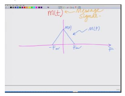
So let us consider a message signal m(t) this is our message signal this is our message signal empty which has the following spectrum let us say m(t) has the spectrum which looks like this that is from minus Fm to Fm, this point is M zero so this is your spectrum M(F) in the frequency domain.
