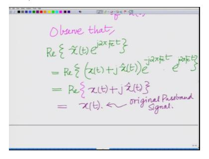
Let us look at this observe that observe observe that if you consider the real part of x tilde t e to the power of j 2pi Fct that will be the real part of, now x tilde t is x(t) plus j x hat of t into e to the power of j 2pi Fct into e to the power of minus j or into e to the power minus j 2pi Fct xet x(t)
