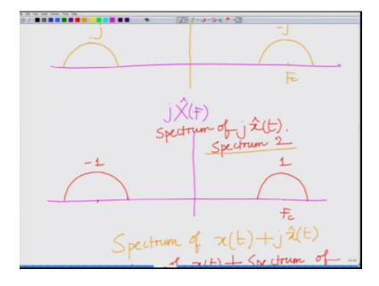
Now spectrum of x(t) is simply both the side bands scaled by one that is unity factor that is the default, now if you look at the spectrum of j x hat of t you can see that the positive band the band that is at Fc is scaled by 1 the band at minus Fc that is the negative band the negative frequency band is scaled by minus 1. So when you add these 2 the positive frequency band that is the frequency bands corresponding to the positive frequencies will add.
