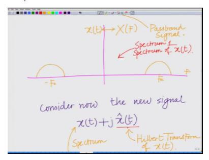
Now the spectrum of x(t) plus j x hat of t, so let us say because this spectrum one that is spectrum of x(t) spectrum 1 this is basically your spectrum of x(t) this is spectrum one.
