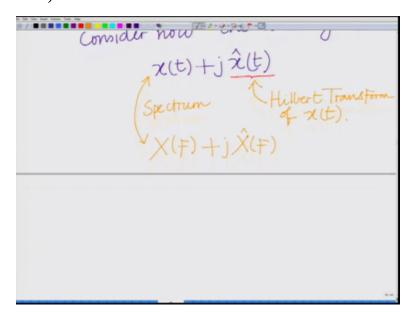
Therefore the spectrum of this signal X(F) will be j X(F) plus times spectrum of x hat of t which is X(F). So this is a spectrum of this. So it's spectrum or Fourier transform of this signal x(t) plus j x hat of t will be X(F) plus j x hat of F, we have already drawn X(F) that is a spectrum of x(t). Let us now see what is a spectrum x hat F going to? What is a spectrum of X(F) plus j x hat? To do that first letter start with x hat of F.
