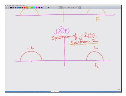
And this is let say spectrum 2, spectrum of j x hat of t, this is spectrum 2, okay. This is so we have spectrum one and we have spectrum 2, alright. And now we have to find the spectrum of x(t) plus j x hat of t, j x hat of t.
