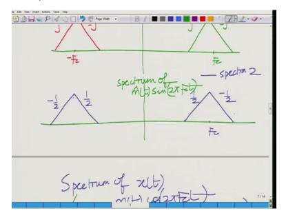
Here the upper sideband in m(t) m hat t sin 2pi Fct upper sideband is scaled by minus half lower sideband is scaled by half therefore you (sub) if you subtract spectra 2 from spectra 1, the upper sideband s will add half plus half the lower side bands will cancel half minus half therefore what is remain?
