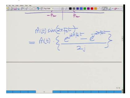
Now m hat of t sgn 2Pi Fct that is modulated by the sgn wave that is m hat of t sgn can be represented as a to the power of j 2pi Fct minus e to the power of minus j 2pi Fct divided by 2j,
