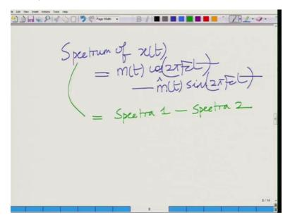
Now the spectrum of x(t) equals m(t) cosine 2pi Fct minus m hat t sin 2pi Fct this spectrum is equal to spectra of 1 that is m(t) cosine minus 2pi Fct minus spectra 2 that is spectrum of and that now if you look at...
