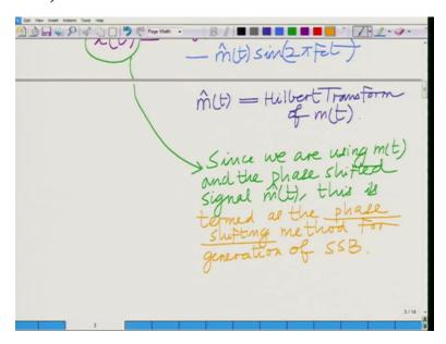
So basically since we are using m(t) and the phase shifted signal and the phase shifted signal m hat of t this is termed as the phase shifting method. A phase shifting method for generation of the phase shifting method for the generation of the SSB signal.
