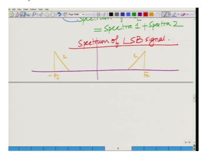
And if you do that you will notice that only the lower side bands only the lower sideband this is Fc the lower sideband only the lower sideband will survive and what you have is, this is basically spectrum of the LSB signal. So this is the spectrum of the LSB signal.
