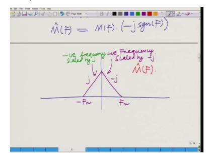
So therefore what you have this is MF original spectrum this is multiplied by minus j sgn F which means that the positive frequency side is multiplied by the scaling factor minus j, negative frequency side is multiplied by the scaling factor, this is remember positive frequency scaled by minus j and phase shifted by minus pi by 2.
