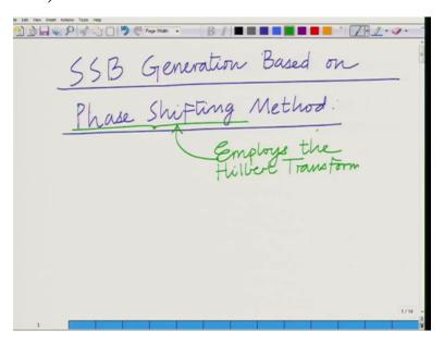
So today let us look at SSB generation using the Hilbert transformer or the phase shifting method which is based on the Hilbert transform is on the phase shifting method, okay. And as we have already said the phase shifting method this employs the Hilbert transform. Now for this purpose considered the message signal m(t), alright with spectrum M(F), okay.
