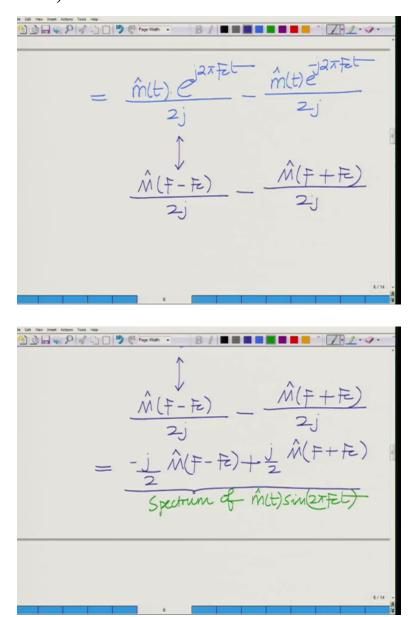
And therefore now this is basically separating this, this is m hat of the e to the power of j 2pi Fct by 2j minus m hat of t e to the power of minus j 2pi Fct divided by 2j and now if I take the spectrum of this spectrum of this is well, m hat of e to the power multiplying by e to the power of j 2pi Fct using the modulation property that is m hat F minus Fc divided by 2j minus multiplying by e to the power of minus j 2pi Fct that is modulation property shifting to minus Fc m hat of F
