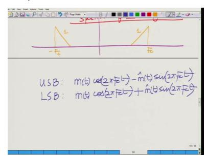
So basically to summarize what we have shown is that the USB signal upper sideband modulated signal is m(t) cosine 2pi Fct minus m hat t sin 2pi Fct and the lower sideband modulated signal is m(t) cosine 2pi Fct plus m hat of t sin 2pi Fc of t and since this employs the phase shifting the
