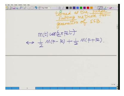
Now let us consider this component by component that is look at m(t) cosine 2 pi Fct, we have already seen this is simply your double band double sideband suppressed carrier signal which has spectrum which is given as the spectrum, so let us look at the spectrum of this that is
