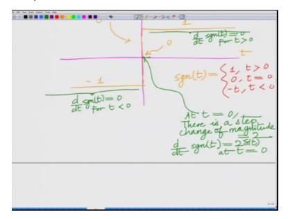
So in this position at t equal to 0 at t equal to 0 there is a step change of magnitude equal to 2 therefore d by dt of sgn t equal 2delta t at t equal to at t equal to 0. Therefore the derivative of this function, so you can see it is constant step change at t equal to 0 and again constant for t greater than or equal to 0, for t greater than 0 therefore the derivative is basically twice delta t, alright. Since the change occurs only at so t equal to 0.
