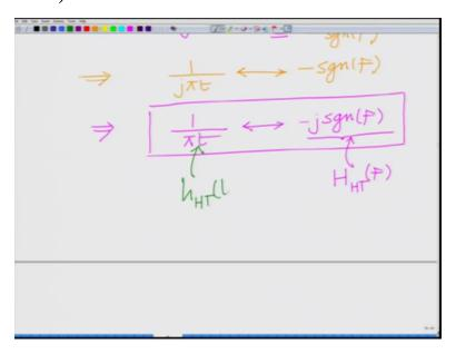
Now taking the j to the other side 1 by pit has the Fourier transform minus j sgn F, 1 by pit has the Fourier transform of minus j sgn F, now minus j sgn F is nothing but recall that minus j sgn F is nothing but the impulse response of the Hilbert transform HHt of F which implies that 1 by pit which is the inverse Fourier transform of this must be nothing but the impulse response of the Hilbert transform therefore the impulse response of the Hilbert transformer is 1 by pi.
