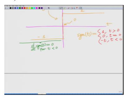
And now you can see the derivative of sgn of t, now here in this region sgn of t that is for t less than 0, sgn of t is constant. So in this region d by dt of sgn of t equal to 0 for t less than 0, right? You can see it is flat. For t less than 0 sgn of t is minus 1. So d by dt the derivative is 0 because it is a constant for t less than zero.
