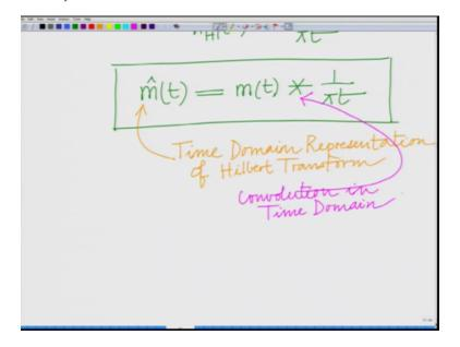
This is the time domain representation of the Hilbert transform this is the time domain representation of the Hilbert transform and this is remember convolution this is a time domain representation therefore it is a convolution in time domain. That is convolution of the input signal with the impulse response.
