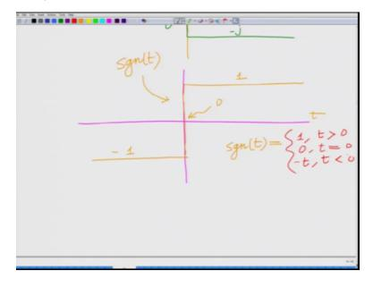
But first let us look at the derivative of the sgn function, let us go back looking at sgn of t, okay. So this is your sgn of t it is one for the greater than 0 minus one for t less than 0 and t equal to 0 it is 0.So sgn of t we already know sgn of t equals one for t greater than 0, 0 t equal to 0, minus t for t less than 0.
