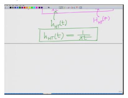
And that is what we have derived H of HT of t equals 1 by pi 1 by equals 1 by pi t, okay. So that is a property that we have been able to show that the impulse response of the, that is if remember the Hilbert transform is a linear time invariant system whose Fourier transform is given by minus j sgn F. In the time domain its impulse response is 1 by pi t therefore now if you look at the Hilbert transform remember the Hilbert transform is an LTI system, correct?
