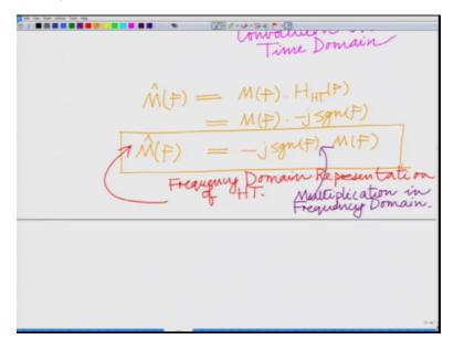
Now frequency domain representation that is the output Fourier transform remember convolution in time domain is multiplication in the frequency domain, so this is MF into H HT of F which is
