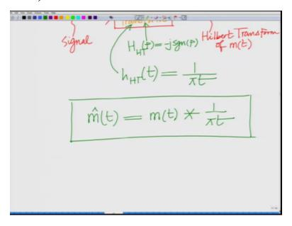
And now the impulse response we have derived the impulse response hHT of t equals one by pit which implies in the time domain the Hilbert transform can be represented equivalently as m hat of t equals the input signal remember when you pass input signal through LTi system signal gets convolved with the impulse response, so m(t) convolved with 1 by pit.
