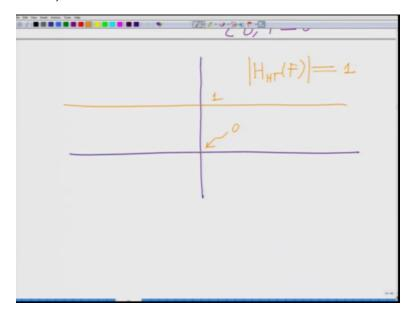
So the magnitude response like this except at 0 where it is equal to 0 except for this single point the magnitude of this magnitude of H the magnitude response of HHT of F is 1 and the phase response.
