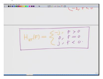
Which means now using the definition of sgn F above the sgn function of F hHT of F equals minus j for F greater than 0 minus j for F greater than 0. 0 or F equal to 0 and j or F less than 0 this is an equivalent expression of the spectrum of the Hilbert transform and therefore now if you look at the sgn function the sgn function looks something like this, so let us first draw the sgn function.
