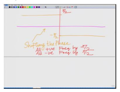
Basically this is what this is doing is this is shifting the Hilbert transform if you can see it is shifting the phase all positive frequencies by minus pi by 2, all negative frequencies by negative frequency components by pi by 2. So this is basically a phase shifter, alright. So Hilbert transform it has a gain of unity and the phase for all the positive frequencies phase shift is minus pi by 2 for all the negative frequencies the phase shift is pi by 2, okay.
