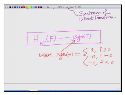
And indeed this spectrum of the Hilbert transform it has an elegant representation that is given as hHT of F is minus j sgn of F I am going to explain what this sgn function is shortly where this sgn function this is sgn of F is literally the sgn function which is one for all positive F that is F greater than 0. 0 or F equal to 0 minus one for F less than 0, so the sgn function sgn of F is
