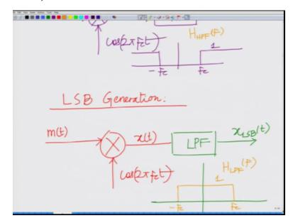
So in practice it is very difficult to design filters with such very difficult to design filters with such sharp cut-off, that is unity for F greater than Fc, 0 for F less than Fc or in the case of low pass filter 0 for F greater than Fc and unity for all F between minus F and Fc. So therefore now that is basically there is no transition band, alright. There is a pass band and there is a stop band and there is no (transi) in practice frequently we have filters have a transition band.
