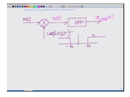
Similarly for LSB generation I start once again with the same signal m(t) this step is the similar for both LSB and USB I modulated with cosine 2 pi Fct to generate x(t). Now at this point pass it through your low pass filter and outcomes the LSB lower sideband modulated signal and again it is not difficult to see that the low pass filter has frequency response that is unity for this is your H LPF.
