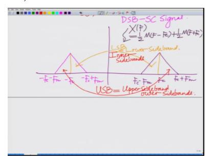
So the lower sideband is comprised of the inner side bands and this USB is the upper side this is comprised of the outer this stands for upper side band and this stands this is basically the outer side bands and now you can clearly see the inner side bands are separated from the outer side bands in the frequency domain. Hence we can use filtering to basically extract either the inner side bands or the outer side bands that is basically the lower side band of the spectrum or the upper side band.
