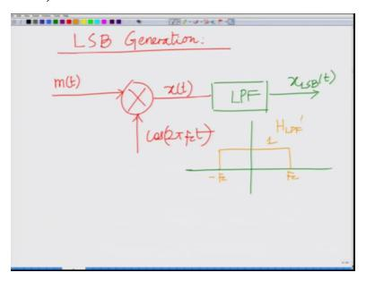
And this is your H spectrum of the high pass filter, the low pass filter has is basically it is an ideal low pass filter as you have seen that the sharp cut-off with a gain of unity for all frequencies within the range minus Fc to Fc. And therefore naturally the question that arises is what happens when these filters are not ideal because in practice it is very difficult to design filters with such sharp cut-offs.
