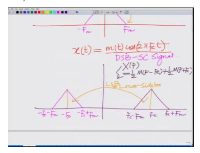
So the DSB SC signal which again we have seen is x(t) equals m(t) cosine 2pi Fct this is also your DSB SC this is your DSB SC signal. The double sideband suppressed carrier signal and this has the spectrum that comprises of 2 bands between centered at Fc so from Fc minus Fm to Fc plus Fm to Fc. So band shifted to Fc and another band shifted to minus Fc so we will have at this is the band shifted to minus Fc.
