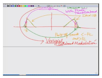
So vestigial sideband modulation is a specially suited for such scenarios so we have vestiges and we have we will see a scheme which is termed as vestigial sideband modulation specific early for such scenarios where it is difficult to design ideal low pass filters and for the same token high pass filter. When you have an non-ideal high pass filter which is a small transition band where it is transitioning from 0 to less than Fc to 1 greater than Fc, alright.
