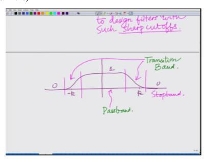
So practical filters have finite transition bands, so practical filters have finite practical filters have finite transition bands and therefore if you pass for instance for the generation of an LSB signal again let us start with your DSB SC signal, correct?
