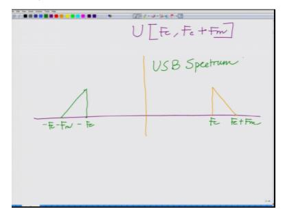
Now let us try to draw these two signals these two spectra separately that is a lower sideband the upper side band and the lower sideband. So naturally the lower sideband spectrum will look as
