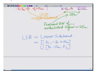
So we have the upper side band and we have the lower sideband just to write it down clearly we have the LSB that is equal to the the lower sideband and that comprises of the intervals minus Fc to minus Fc plus Fm Union together with Fc minus Fm to Fc this is the lower sideband that is minus Fc to minus Fc plus Fm to Fc minus Fm t Fc.
