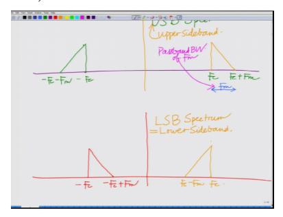
And now you can clearly see that both USB and LSB if you look at the pass band bandwidth of both USB the USB pass band bandwidth is from Fc to Fc plus Fm which means it has a pass band bandwidth of means this scheme has a pass band bandwidth of Fm and similarly the LS LSB signal also has a pass S Fc minus Fm to Fc that is it has a pass band bandwidth of Fm.
