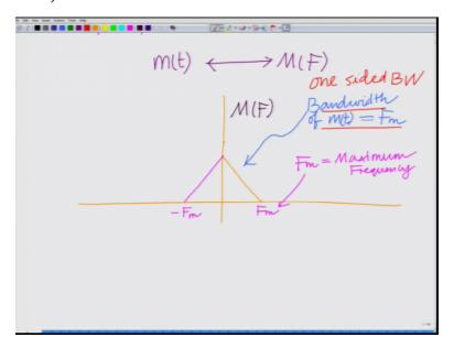
We have an message signal m(t) and it is Fourier transform given by M(F), okay. Let us draw this schematically over here we have our message signal we have our message signal m(t) I am drawing the Fourier transform, so let us say the Fourier transform is between minus Fm it is minus Fm to Fm where Fm equals the maximum frequency of or the maximum frequency component correct?
