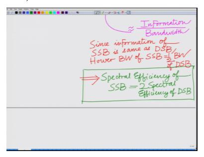
Therefore the spectral efficiency of SSB spectral efficiency equals twice the spectral efficiency of DSB that is double sideband modulated signal and this is an important result. So SSB is a very important scheme or it is a very efficient scheme because it results in a significant reduction band with precisely how much reduction in bandwidth (reduc) leads to a decrease of leads to a decrease of the DSB bandwidth by a factor of half, alright.
