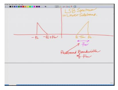
So it has a pass band signal it has a pass band bandwidth of Fm. So you can clearly see that the double sideband suppressed carrier signal has a pass band bandwidth of two FM where both the
