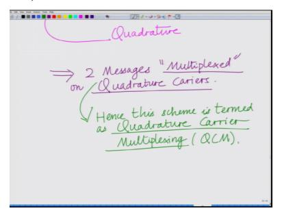
We have 2 messages which are multiplexed on quadrature carriers hence this scheme is termed as quadrature carrier multiplex this scheme is termed as quadrature carrier multiplexing which is abbreviated as QCM scheme will be transmitting 2 message signal is different message signals mIt mQt on quadrature carriers is termed as quadrature carrier multiplexing further notice an interesting property of these quadrature carriers notice an interesting.
