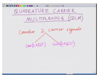
So we want to start looking at quadrature carrier multiplexing that is QCM. Now for this purpose consider there are 2 carriers or 2 carriers. Consider the carrier signals let us consider the following 2 carrier signals that is cosine 2pi Fct which is the standard carrier signal at carrier frequency FC and also now sin 2pi Fct, so these are our 2 carriers that is cosine 2pi Fct and sin 2pi Fct and Fc as usual is the carrier frequency.
