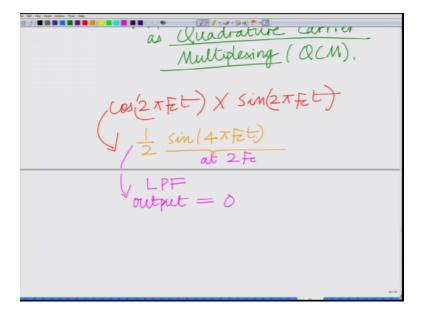
Consider now for instance let us say we multiply or demodulate cosine 2pi Fct by sin 2pi Fct that is we are multiplying at the receiver by sin 2pi Fct demodulating uhh cosine 2pi Fct by sin 2pi Fct that gives half sin 4pi Fct which is basically at 2 (freq) 2 times a carrier frequency 2Fc therefore if I low pass filter this LPF if we pass it through a low pass filter the resulting output equal to 0.
