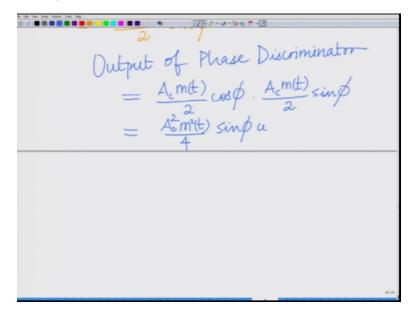
So output of phase discriminator so let us write this down output of the phase discriminator equals Ac m(t) by 2 that is product of the outputs of the low pass filter on the upper branch and
