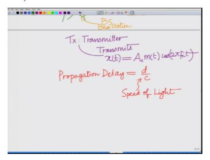
Now let us assume that this distance of propagation this is the propagation distance this is the propagation distance, okay. And let us say the transmitter that is the transmitter transmits signal or transmits the signal x(t) equals m(t) alright let us go back and let us say this is  $Ac\ m(t)$  cosine  $2pi\ Fct$  this is a signal that is transmitted by the transmitter, now the propagation distance there is a distance between the transmitter and the receiver.
