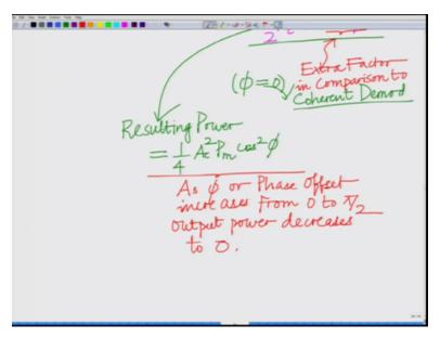
Coherent demodulation means phi is equal to 0 and power the resulting power equals 1 over 4 Ac square the power in the message signal times cosine square phi which becomes progressively worse as phi which means as phi increases that is as phi increases as phi increases from 0 to pi by 2 or as the phase offset as phi or phase offset increases from 0 to pi by 2 output power decreases to 0. So the performance becomes progressively worse, alright. This is what we have seen, alright.
