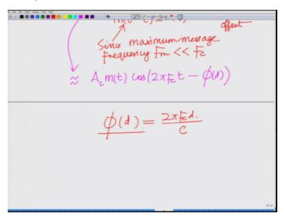
Since the message is varying since the maximum message frequency Fm is much lower than Fc, correct? Since maximum message frequency Fm is much lower than Fc, correct? Since the maximum message frequency Fm is much lower than Fc I can say therefore that this is approximately equal to Ac m(t) cosine 2pi Fct minus d by minus 2pi Fc d by c minus let us write this as the phase phi which now depends on the distance d the phase phi phi of d equals 2pi Fcd by c.
