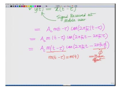
And therefore signal received at the receiver signal received at the mobile user the signal received at mobile user is y(t) which is x(t) minus Tau that is remember delayed version of x(t) and naturally signal x(t) minus Tau implies basically the signal x(t) delayed by tau and therefore the signal y(t) is now if you substitute for x(t) this is Ac of course Ac is a constant x(t) minus
