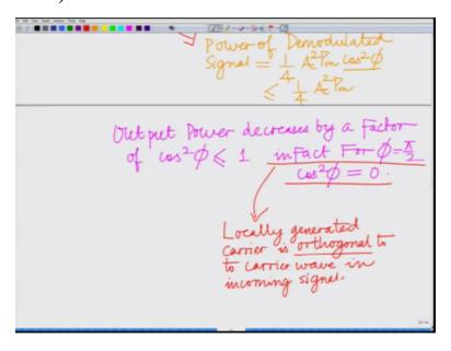
So output power the output power decreases by factor of cosine square phi which is basically less than or equal to 1 in fact for phi equal to pi by two cosine square phi equal to 0. In fact if the phase difference phi is pi by two that is a locally generated carrier is phi by two out of phase with respect to the carrier wave in the incoming signal the output power is 0 as you low pass filter it, right?
