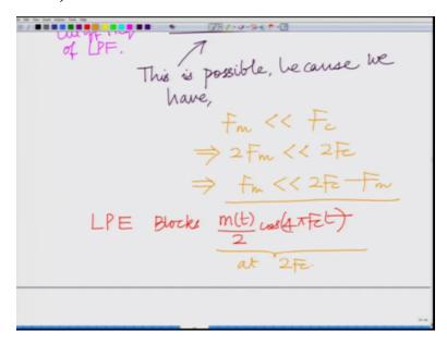
So the LPF basically LPF blocks the component cosine two pi Fct m(t) by two cosine four pi Fct, this is the component at two Fc, right? The carrier has a common frequency cosine corresponds to cosine four pi Fct corresponds to the frequency two Fc, alright. So in this module what we have seen is we have seen a new form of amplitude modulation that is double sideband
