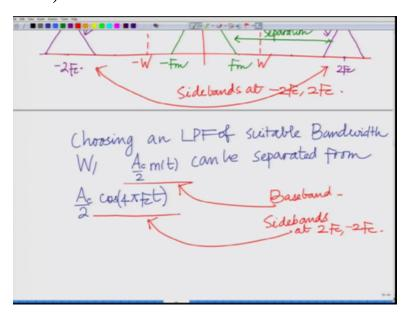
So choosing a low pass filter of bandwidth W LPF of bandwidth of let us say suitable bandwidth. Let us make it suitable bandwidth W Ac over two m(t) can be separated from Ac over two cosine four pi Fct, correct? Because this is your base band this is in the baseband and this is actually these are the side bands at two Fc, minus two Fc.
