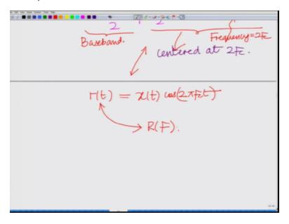
So let us look at the spectrum to understand this better let us look at the spectrum, so the spectrum of this that is r(t) equals x(t) cosine two pi x(t) multiplied by the coherent carrier and if I look at the spectrum of this that is R(F) I can draw it as follows.
