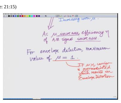
So now you observe this implies as Mu increases efficiency eta of AM signal increases this is important to remember as mu increases the efficiency increases. Now however interestingly mu remember for envelope detection the modulation index mu has to be less than or equal to one if mu is greater than one the signal becomes over modulated therefore for envelope detection mu has to be the maximum value of mu can take is one.
