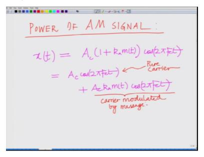
Power of amplitude modulated that is the AM signal and we know that a typical AM signal is given as s(t) or x(t), let us use the notation x(t) equals A cosine or basically Ac one plus ka m(t) into cosine two pi Fct which is the carrier component Ac cosine two pi Fct plus the message component that is AA Ac that is a carrier modulated with the message that is Ac ka m(t) cosine two pi Fc of t, correct?
