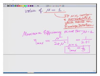
Maximum efficiency occurs which means eta max equals mu square by two plus mu square evaluated at mu equal to one which is one by two plus one which is one over three, alright. So this is eta max.
