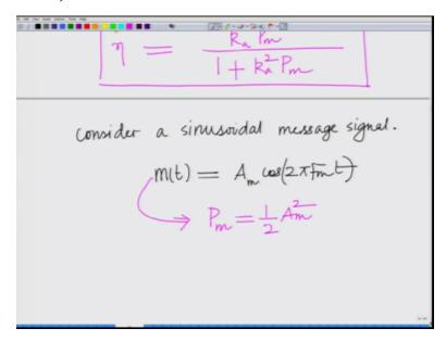
Consider now the specific case of a Sinusoidal message signal, consider a Sinusoidal message signal m(t) equals Am this is our message signal with amplitude Am cosine two pi Fmt, alright. Therefore this implies that the power of the message signal Pm equals half Am square.
