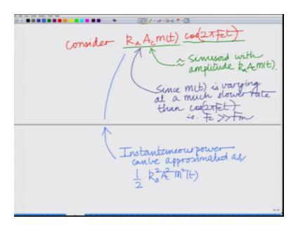
So now consider the other component that is Ka Ac m(t) co sine two pi Fct now you can think of this as the carrier and this as the amplitude that is you can think of this although this is not exactly correct you can think of this as Sinusoid with amplitude that is I am writing using the approximate signs Sinusoid with amplitude ka Ac m(t). Well, correct? Although strictly speaking that is not true because when you multiply m(t) time varying signal m(t), correct?
