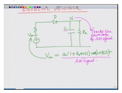
This is our input signal which is our Am signal is fed as input to this and we said this is the envelope detector and the V out, correct? Tracks the envelope tracks the envelope of the AM, this tracks the envelope of the AM signal and we have said that if I denote this RIC, correct? This time constant Tau equals RIC, correct? This is the time constant of the envelope detect, correct?
