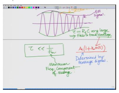
So Tao very large, so Tao equals RIC, correct? Tao equals RIC very large implies fails to track the envelope, correct? And in particular remember the envelope is determined by the message signal the envelope is basically one plus ka into m(t) envelope that is the rate at which the envelope is changing the envelope the rate at which this envelope is changing is determined by the message signal. So this is determined by your message signal, correct?
