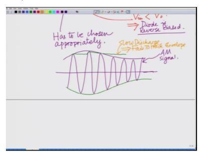
Let us consider an amplitude modulated signal, right? Correct? This is your AM signal which is fed as input to the peak detector, now we have when it is fed as input to the envelope detector the capacitor charges, correct? And it discharges now if the time constant is very large then the discharge is going to be very slow and what might happen is once it charges the discharge is so slow that it fails to track the variation of the message.
