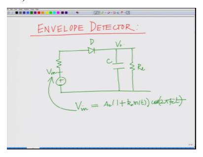
So let us continue our discussion on the envelope detector and we have seen that the envelope detector is a very simple circuit, correct? The amplitude modulated wave is fed as input it comprises of a diode, correct? And a capacitor a capacitor and a load resistance in parallel, so this is correct? This is output this is the input voltage and we have said that the input voltage is our AM wave that is Ac one plus ka m(t) times cosine two pi Fct this is our amplitude modulated signal, correct?
