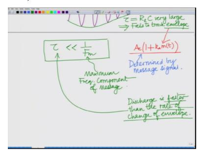
So that means basically time period, so discharge is faster so this implies discharge if time period discharge is faster than rate of discharge is faster than the rate of change of the envelope the rate of change of because the envelope remember is proportional to the message signal which is changing, alright. Which is changing at the rate uhh that is the rate Uhh that is basically it is
