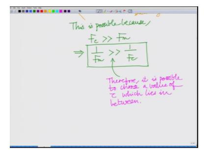
And finally also note that this is possible because note that the interesting point to note here that this is possible only because the carrier frequency Fc is much greater than the maximum message frequency Fm which implies one over Fm is much greater than one over which implies that one over Fm is much greater than one over Fc and therefore it is possible to choose a value of Tao which lies in between.
