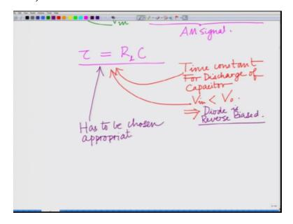
This is the time constant for discharge, correct? Once the diode of one's the diode is cut off that is when the output voltage of the capacitor is when the capacitor reaches the peak in the input
