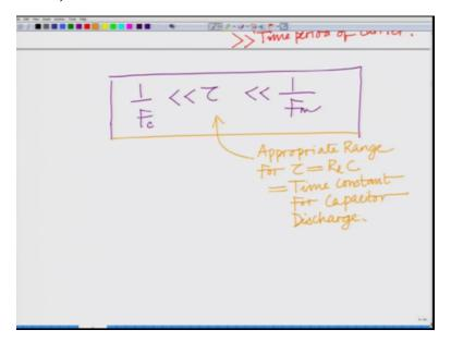
And now combining these two conditions we have Tao must be less than one over Fm and it must be greater than one over Fc, correct? So this is basically this is the gives the appropriate, this basically gives the this basically gives the appropriate range for Tao this is basically gives us the appropriate range for (ti) Tao equals to RIC which is basically your time constant which is the time constant for capacitor discharge.
