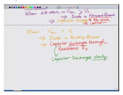
So the so the envelope detector works on the principle basically the principle of envelope detector a is when a when your AM wave that is equal to V in is less than Vo this implies diode equals or when V in is less less than Vo or when V in is greater than Vo the input voltage is greater than or equal to Vo. Diode is forward biased, so this is your so this is your diode let us
