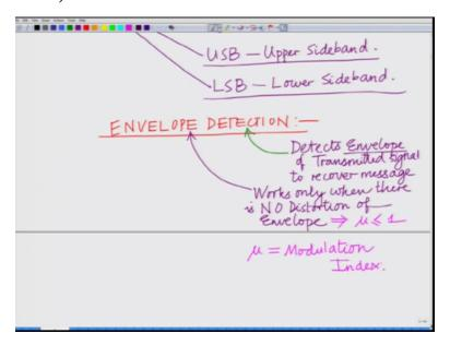
Now let us look at detection for this AM signal or amplitude modulated signal and one of the most popular schemes for detection is what is known as envelope detection and as the name implies as the name implies envelope detection detects the envelope, correct? This detects the envelope this detects the envelope of the transmitted signal to recover the message.
