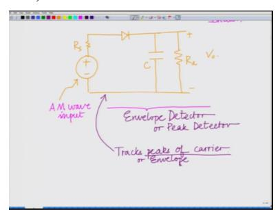
Envelope detection employs a single circuit which is known as the envelope detector and that can be explained as follows I have an input here, alright. And this is my source resistors Rs I have a diode, correct? A capacitor with charges and discharges and a load resistance Rl and I measure the voltage V not across the capacitor, correct? So no this is known as this circuit and the AM wave is given as input, the AM wave is given as input to this circuit, alright.
