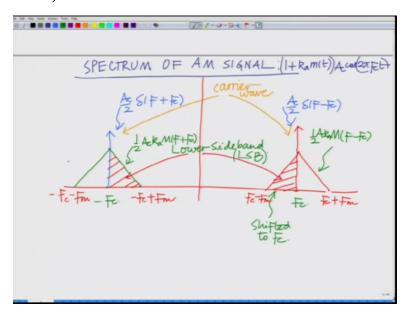
So what we are going to have net is basically now we are going to have the spectrum which looks as follows we are going to have at at Fc we are going to have MF minus so this is basically your MF shifted to Fc that is M(F) minus Fc half Ac ka that is this is basically your shifted to Fc, correct? Correspondingly over here we are going to have the image that is shifted to minus Fc, okay. So this is half Ac this component is half Acka M F plus Fc plus if I add the spectra of the carrier.
