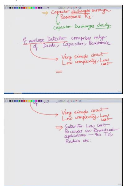
So this is envelope detector to add the envelope detector comprises only of a diode, a capacitor and resistance, correct? And therefore it has a simple circuit suited its very simple circuit and it has a low complexity and low-cost more importantly it has a low complexity and therefore this is suited for development of low-cost low-cost receiver low-cost receivers such as televisions or radio sets in especially broadcast applications, examples being your TVs or transistor sets or radio sets etc.
