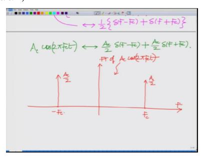
And therefore Ac if I multiply this by Ac that is Ac cosine two pi Fct this has a Fourier transform Ac cosine two pi Fct has the Fourier transform Ac by two delta F minus Fc plus Ac by two delta F plus A Fc and therefore if you draw the spectra of this part that is the carrier it comprises of two impulses Ac by two at Fc and another impulse scaled by Ac by two at minus Fc, correct? So this is the Fourier transform or Ft of Ac, this is the frequency axis, okay.
