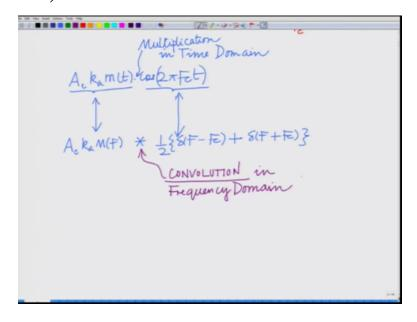
Now let us look at the other components that is Ac ka, so observe Ac ka m(t) times cosine two pi Fct. Now this is a multiplication in the time domain, now Fourier transform of Ac of this part will be Ac ka M(F) Fourier transform of this part will be half delta F minus Fc plus delta F plus Fc Fourier transform of cosine two pi Fct is half delta F minus Fc plus delta F plus Fc plus the two signals are multiplied in the time domain which means the respective spectra will be
