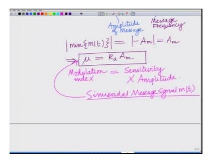
And finally for a Sinusoidal message signal, for a Sinusoid message signal, correct? We have m(t) equals Am times cosine 2 pi Fmt this is amplitude of your message, this is the message frequency, correct? This is the message frequency and you can see magnitude minimum m(t) the minimum value of Am cosine 2 pi Fmt is - Am, so magnitude minimum m(t) is Am is positive that is magnitude minimum Am which is Am, correct implies Mu equals ka times Am, correct?
