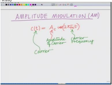
So let us start looking at amplitude modulation which is an analog communication scheme and one of the earliest communications schemes developed and widely used, this principles continued be used even today that is amplitude modulation often abbreviated as AM. Now any communication system or communications scheme involves a carrier signal which is a Sinusoidal signal, alright.
