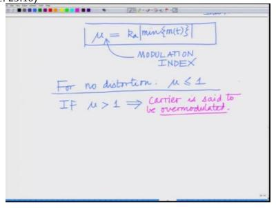
The modulation index of this amplitude modulated system mu equals ka times the magnitude of minimum of m(t) where mu is the modulation index of these amplitude modulated system. Now
