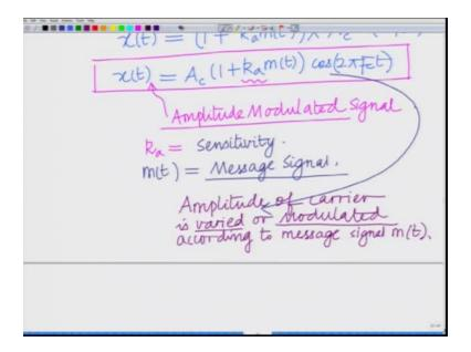
So in amplitude modulation so what we have in AM is basically your amplitude of the carrier. That is message modulates the amplitude of the carrier and an AM signal is given as the AM signal is described as x(t) which is equal to 1 plus ka let me write the expression 1 plus ka m(t) times the carrier that is Ac cosine 2 pi Fct which is also basically Ac plus 1 plus ka times m(t) into cosine 2 pi Fct. This is the standard form or the canonical form of the amplitude modulated.
