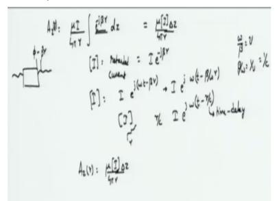
Substitute for J of r-prime dv-prime as I delta z z-prime, okay. So, I have mu by four Pi, so I have mu by four Pi, and this r would be the radial distance r that we are considering, because it is so small that I can simply push this one out. So, I have mu I by four Pi r, and there is e to the power minus j beta r and there is integration along dz, right. So, this is what I have, of course, what I have this e power minus j beta r is nothing the retarded value of I.
