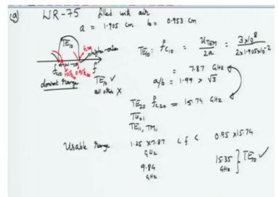
Let us try to solve one problem before we go on to the next topics in the waveguide, we want to consider a waveguide, which is widely used, which is called as WR-75 waveguide okay, this numbers are just a numbers, which would tell you the ratios of a and b. For this waveguide, which is filled with air, so the waveguide is filled with air, which means that mu is equal to mu zero and epsilon is equal to epsilon zero.
