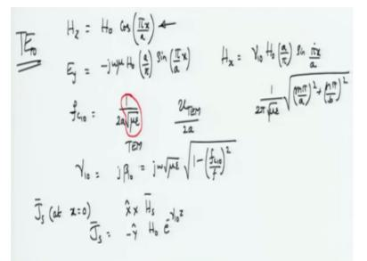
For the TE one zero case, the HZ component will be some constant H zero cos of pi x by a right. All the dependants on y is gone. There would e to the power minus gamma m n z that can be written as a common factor. If you go to Ex, you will see that Ex will be equal to zero because that would correspond to differential of HZ with respect to y whereas you will have Ey component that is non-zero.
