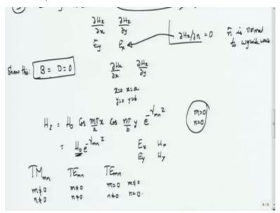
The up short of all this very hand waving analysis is that, at each of the waveguide walls we will apply the derivative condition okay or the normal condition. So del HZ by del n equal to zero where n is the normal to the wall okay, normal to waveguide wall. The philosophy behind the normal derivative of HZ being equal to zero is simply that these normal derivatives will determine the electric field components, which will be tangential to the appropriate waveguide walls.
