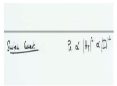
So, let us obtain the surface current because surface current will determine for an imperfect conductor. Surface current is required in order to find out how much power is being lost because of the conduction. If you remember our discussion on skin depth, we wrote something like this, 'the power dissipation per unit area' was something that was proportional to magnitude of 'H T square', where 'H T' was the transverse component for the corresponding conducting surface.
