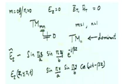
In the TM mode case, the functional forms are 'sin m' and 'sin n', if I put 'm' is equal to zero, 'n' is equal to zero, in the hope of obtaining the lowest order mode, I will not be able to obtain anything. Because for 'm' is equal to zero and 'n' is equal to zero, 'E z' will be zero, which also makes the total electric field, the transverse components and that magnetic field transverse components also go to zero.
