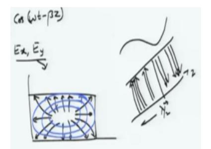
And we can see that the field lines, here there won't be, at the center it would be very small. So, at the center I am actually not plotting like this. So, it would be in this way. So, let me remove this center lines as well. So this we have removed the center. So this is how electric field lines would look. The electric field line does not have any value at the center because if you remember that becomes cos and then in the middle there would be a symmetry.
