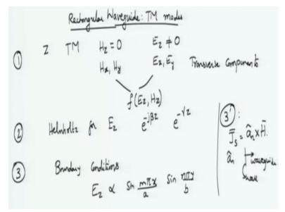
In the last module, we were discussing rectangular waveguides and we discussed how to derive expressions for transverse magnetic modes. If we recall what transverse magnetic modes are, these are the modes for which the magnetic fields lie entirely in the plane that is perpendicular to the direction of propagation. Because, we have chosen Z as the direction of propagation, this statement TM mode simply means that there is no H z component.
