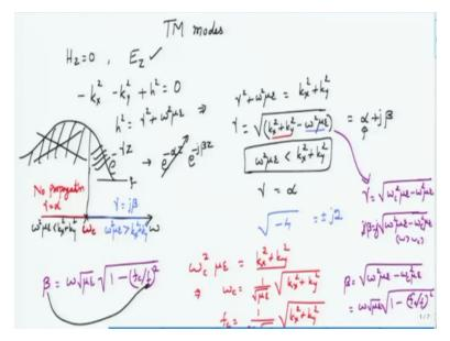
It means that if you have a frequency spectrum, so far some way you have a pulse, which is to be propagating inside, then if the frequency components are all lying, you know some frequency components lying below 'omega c', they would all be filtered and cancelled out or they would be attenuated out. Only the components, which are greater than 'omega c' will be allowed to propagate.
