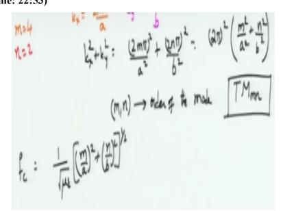
So 'F c' is this fellow 'm / a whole square + n by b whole square' under root. So this is the expression for cut off frequency. So we still have to figure out what is 'E z' completely. We have figured out what is 'E x' the 'y' dependence, 'E y' the 'x' dependence, the 'z' dependence is
