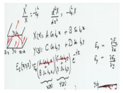
Go back to the picture of the cross section. In this case, may be the cross section does not really help. So you need to write down the wave itself. You will have this scenario. So, this is your wave equation. So, you actually have two conductors here or it seems that you have two conductors, one is at 'x equal to zero' and one at 'x equal to A'. And you have two bottom conductors, one at 'y equal to zero', one at 'y equal to B'.
