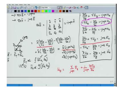
Now, how do we do that? Consider for example, the second equation, okay. So, let me highlight that equation, okay. I use this equation to solve for H y. What do I mean by that? I simply take this minus j omega mu on to the left hand side and then write down what is H y, okay. So, you can see H y is actually equal to gamma by j omega mu E x, okay, by taking minus one by j omega mu down and you have also plus one by j omega mu del E z by del x.
