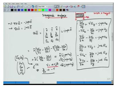
So, if you look at the cross section this is how they would look probably let us make it more rectangular rather than square. So, along x axis, along y axis, the width of the waveguide is a and the height of the waveguide is b, okay. In the traditional notation, the width is actually taken to be larger than the height, okay. And, we will see why that has to be done. Although in principle there is no difference between width and height.
