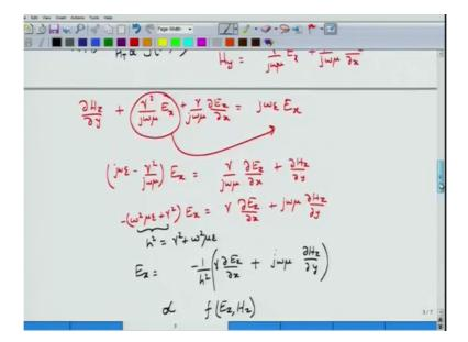
So, let me use that equation and write down substitute for H y, so what do I get. I have del H z by del y that hasn't changed, right, plus gamma square by j omega mu E x plus gamma by j omega mu del E z by del x must be equal to j omega epsilon E y, right. So, with this I can actually pull this gamma square by j omega mu epsilon to the, sorry, this is actually E x, right. So, this is E x not E y, okay.
