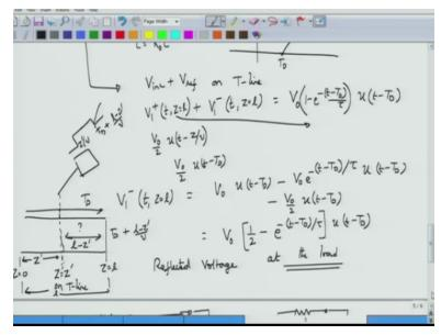
So, capacitor voltage V L of t is given by V L of infinity V 0, V L of zero is zero and tau is R 0 C. So, V L of t the capacitor voltage will be equal to V 0 into 1 minus e power t/ tau. So, this is how the load voltage would look like. So, this would of course start at T equal to T D and therefore you need to account for that one as well. So, this is the load voltage across the capacitor and this is how it would behave.
