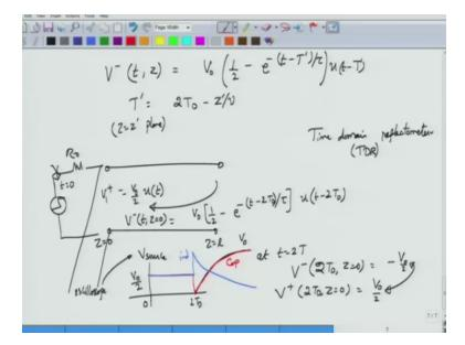
Which is v minus at t for any value of z will be equal to V 0 into 1/2 minus e to the power minus t minus t prime. It is the time at which the plane, the oscilloscope at z equal to z prime sees a change in the voltage divided by tau. So, nothing has changed over her except that the time is not exactly the same. So, T prime is actually equal to two times T D minus z prime/v. You can see that this is correct.
