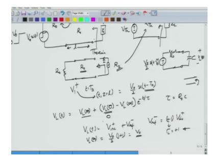
Well, I have this source side R 0 with this V 0 u of t at the switching way form and then I have a transmission line which also has a characteristic impedance R 0 and then I have this load. So, in this particular case the load happens to be a capacitor it could be any capacitor. What I want to do is, I want to find the Thevenin Equivalent at this point. What would the Thevenin Equivalent look like?
