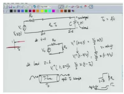
This is a situation where the driver connecting the load and via a termination line is actually driving a capacity load something that you would see when a CMOS is pulling up or pulling down and it is driving one more CMOS which will of course pull down or pull up in response to the initial CMOS invertor. And on a printed circuit board or on a computer motherboard you would actually see lot of these circuits.
