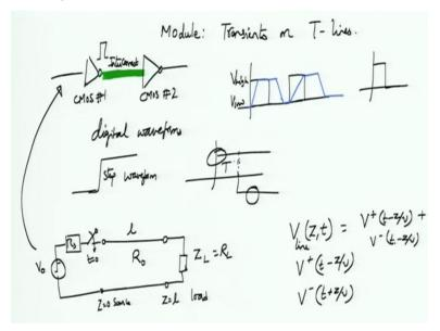
In this module we will look at transients on transmission line. From the earlier modules on transmission lines we considered sinusoidal excitation that is we took sinusoidal voltage source of a particular frequency or a given wave length connected that to a transmission line circuit that could have loads that could have different links different characteristic impedance all these things we saw.
