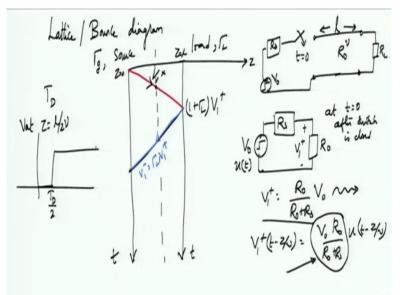
The way to analyze these transients or this digital step waveform on the transmission line is to write down what is called as lattice or bounce diagram okay. This is a nice graphical approach of course more complicated analysis has to be carried out numerically but for this course we will assume that things are simple and we will understand how to use this lattice or bounce diagram. If nothing else this will at least tell us how to actually approach the problem.
