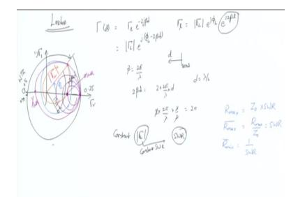
So going back to representation of gamma l on the plane this would correspond to gamma r and this is the imaginary j gamma i, so you draw a line okay of length magnitude of gamma L which would be the load reflection coefficient and the magnitude of gamma L would essentially the same, okay. This initial angle will be phi L okay so that you are actually representing this gamma L magnitude e to the power j phi L.
