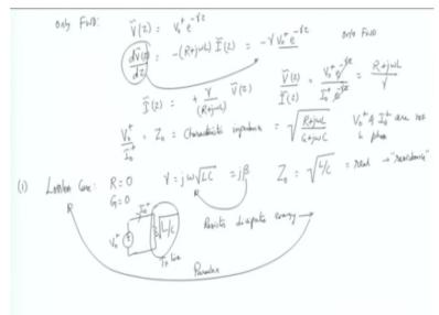
So let us for now assume that there is only forward going wave okay. So let us assume that only forward going wave is there which means that the voltage phasor is v zero plus e power minus gamma z and then differentiating this voltage phasor and equating it to the current term, what you get is minus R plus j omega L into I of z. So this equation, when you differentiate this v of z with respect to d z, will give you minus gamma v zero plus e power minus gamma z.
