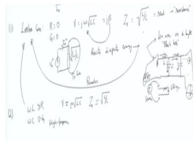
For now, we are considering only forward going wave, which means that there is no end to the line. The line was actually infinite right. So line was actually infinite in length or it was matched with z zero will come to matching thing later. For now, we will assume that this line is infinite in length and for an infinite length, if the voltage source connected at the input terminals of a transmission line generates a certain current.
