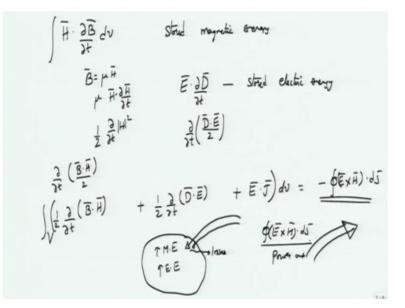
What about the term that you have as H dot del B by delta t integrated over the volume. This term is actually the stored magnetic energy, okay? Why again go back to the circuit kind of an idea, B is equal to mu H, right? So this H dot del B by del t would give you something like H dot mu can come out delta H by del t, right, or you can replace this one by del by del t of magnitude H square half, so half of del by del t magnitude of H square.
