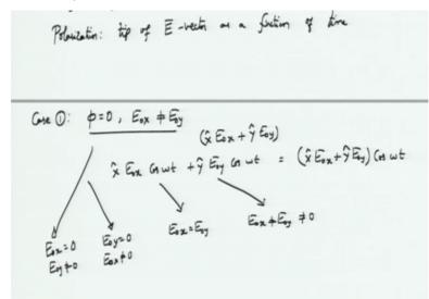
Polarization can be defined in many ways. One most common way is to actually look at this as tip of the electric field vector as a function of time, okay? This is called polarization. So what we were saying was, the electric field have two components, x and y and there would be a relative phase difference between the two which is captured in the form of this angle phi and then fixing up a particular plane.
