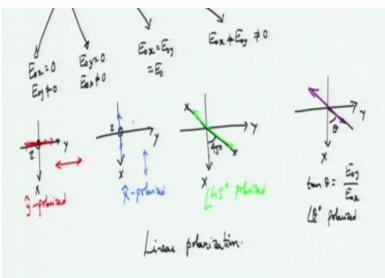
So if you draw the x and y axis in this way, there is a reason why I am drawing it in this way, I will tell you. You are looking from the top, right, you are looking from the top along the z axis, this is the direction in which the wave is approaching you and you are looking from how the wave is actually approaching you, okay?
