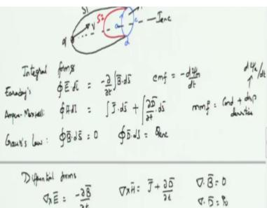
So, we have Faraday's law, what is Faraday's law? The EMF induced right, which is given by the integral of E over a certain loop, must be equal to minus del by del t integral of B dot d s. Remember Faraday's law, actually has two types of relation right, one where the path is varying and one where the field is varying but both are the essentially equivalent right, in words this would be EMF induced is equal to minus d psi m by d t, where psi m stands for magnetic flux okay.
