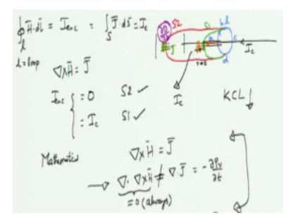
Whatever the current that is enclosed by that closed contour so let us call this contour as some L okay, to indicate that this is actually a loop. I could have used C, but I have already used C for capacitor. So, I do not want to confuse two C's. So, I am using this L to stand for loop okay. (Refer Slide Time: 14:00)
