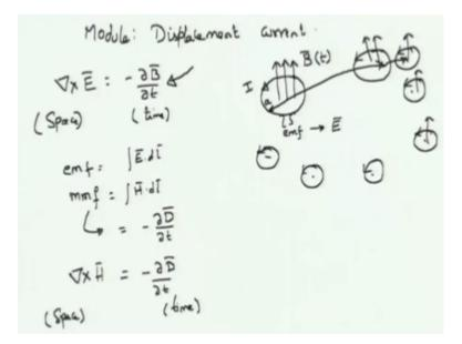
And we expressed this Faraday's law in a compact form by writing this as curl of electric field would be equal to minus del B by del t. This was the point form for Faraday's law. What is the physical meaning for this one? Physically it means that, you can consider a loop okay, almost a closed loop is what we are considering and when you let the magnetic field passing through this loop change with time right.
