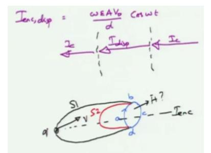
When i do that i see that this is simply since this is perpendicular to the surface, this would corresponding to simply multiplying this one by the total area a right. So this expression the total current, which would be because of the displacement would be equal to omega epsilon A V 0 by d cos omega t and if you see what is that we have return earlier, this is exactly the same current the charging current IC that we have obtain here.
