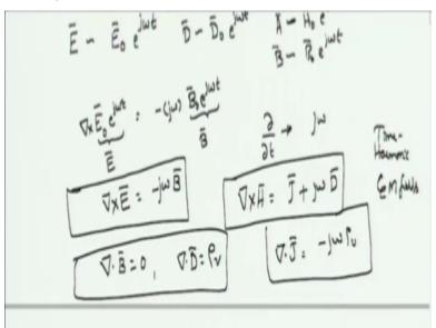
There is one additional form of these equations which are useful for us okay and this additional form results when we assume the time variations of the electric fields in the form of a facer. What do I mean by that if the electric field let us say has certain value is E 0 right, it is pointing a certain direction E 0 but with respect to time, it is changing has some sin or cosine or in general changing has e to the power J omega t right?
