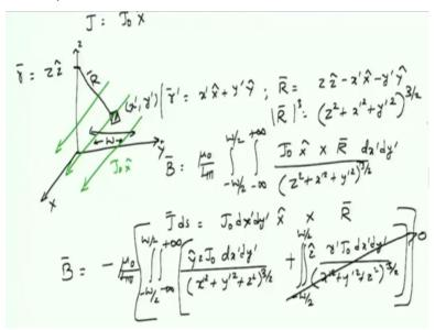
Now apply Biot-Savart law and write this as integral from some width over the Y direction. And for the X it would be from - infinity to + infinity. The current directions are all constant and they are all going from - infinity to + infinity along X axis. Whereas for Y, I am considering a strip of
