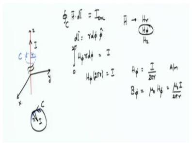
Let us assume that we have a wire which is carrying a current I. This current I is supposed to be uniform and the wire extends all the way from - infinity to + infinity. Let us orient this wire along the z axis of the Cartesian coordinate system. So, I have the z axis along which the wire is extended or the wire is placed and the wire of course goes all the way from z equals - infinity to + infinity.
