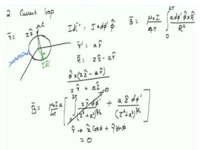
So we were discussing in the last module about finding the magnetic field or the magnetic flux density of a current loop and here is this half thing that we have done. So we have a current in the form of a loop of radius a. And then we wanted to find the field on the axis of this loop at a distance of Z from the loop itself. And we wrote down this integrals I dl prime was I a d Phi prime along the Phi axis.
