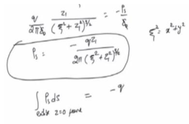
So this is zeta square, right, at Z equal to zero, if you find this out, you will see that this would be q by there is a two in the numerator, four in the denominator, so this becomes q by two pi epsilon zero Z1 divided by zeta square plus Z1 square to the power three by two. Why, because Z equal to zero so minus Z1 square is as good as Z1 square, so you can actually combine this equation and find that Z cancels with each other, and you are left with only Z1.
