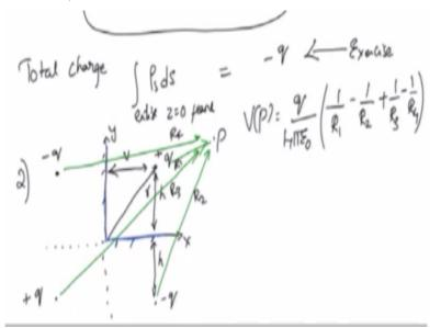
Let us consider a second example of images, we will not be giving you the entire solution here. The idea is to just see how to extend this solution, okay. Consider two conductors which are bent, such that they form right angled corner, okay. They form these corners in the entire quadrant with x greater than zero and y greater than zero, okay. So these are the conductors, okay, and now I place a point charge here, okay.
