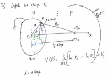
Now, we will solve one more image problem, this is important in the practical sense. They have actually used the results of this, without really telling you where we have used it. But you will soon recognise that one. Suppose I have an infinite line charge, okay, I have an infinite line charge, okay, positively charged with a charge density rho L. And I take grounded conductor, okay, I take a spherical grounded conductor over here.
