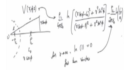
So if the positive line charge is at L0 on the x axis, now the negative line charge is at minus rho L, note that I have removed the conducting cylinder that is not really required now, but my solution has to be extended or valid only for the region greater than a, okay. So this is where the original cylinder was located, the grounded cylinder was located, okay. This is the origin.
