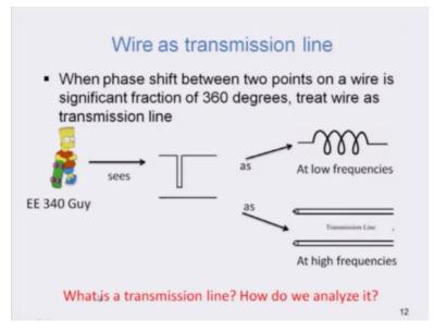
So that leads us to the question as to what is a transmission line, and how do we analyse this transmission line.
