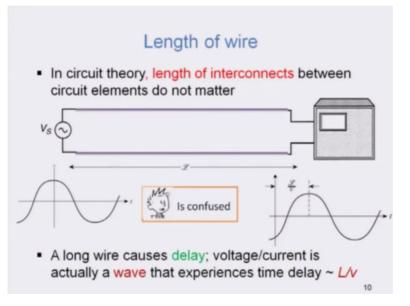
Finally, we come to the length of the wire, okay. In circuit theory again length of a wire or a interconnect between two gates or two circuit elements does not really matter. It could be any length, but what we assume is that the voltage at one end of the wire or the interconnect is exactly same at the other end of the wire, right. So that is if you can take the length of the wire to be say, one kilometre, two kilometre, three kilometres, that does not really matter.
