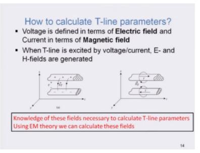
Again we have to go back to electromagnetic theory to understand where these parameters are coming from. For example, if you want to calculate the characteristic impedance, if you remember the impedance definition, the impedance definition is voltage divided by current. However, we have seen that voltages and currents are not just numbers, they are dependent on where you are measuring them, right.
