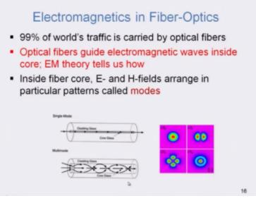
It is not just circuits where Electromagnetics comes up often, it is also that electomagnetics opens up a wide array of topics that one can specialize in, that is one can find applications of Electromagnetics in. Now, you must certainly have heard about fibre optics and optical fibres are the ones which can carry 99 percent of the world's traffic, right.
