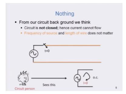
From our circuit background, we might first think that well circuit is not closed, which means that there cannot be a current flow in the circuit. Whatever the voltage that is there at the source end will directly be available at the load end, right. The open circuit voltage of the source will be equal to the voltage at the load end. Now frequency of the source and the length of the wire does not really matter to us.
