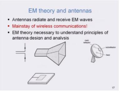
Now you might go to antennas or radars, in radars antennas are one of the major components and in wireless communications antennas are there everywhere, right. Without an antenna, one cannot have wireless communication possible, now to understand how there, I have shown different types of antennas over here. This is simple dipole antenna, this is a horn antenna, this is a reflective antenna, and this is micro strip antenna.
