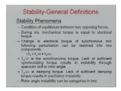
So, the stability general definitions, let us see what is the stability phenomena. Basically the stability, is can be defined, can be understood by looking at the condition of equilibrium of two opposite forces. So, stability phenomena, basically can be realize by understanding the condition of equilibrium between two opposite forces, to understand this, here for any system here.
