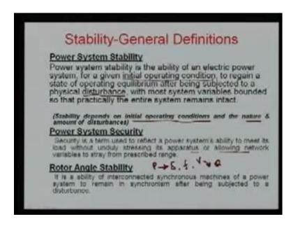
So, if your monitoring quantity is your angle, then it is called your rotor angle stability. Means monitoring means what, I am just going to say means this parameter is more concern, than other these two parameters, then we can say this is rotor angle stability. And you know this rotor angle stability is directly angle, here this is related with directly
