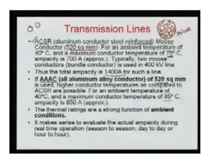
This ACSR as I mentioned it is aluminum conductor steel reinforce, means what we do we use the steel inside, and around this we use the aluminum conductors, and it is called; means there may be not only one layer of steel, it may be the one or two layer of steel and over and above we can go for here the aluminum conductors. So, normally this type
