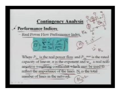
So, you can say this omega m or real non negative weighting coefficient, which may be used to reflect the importance of the lines. Here, in the contingency analysis, just I have set the performance index based method; I am using the real power flow performance index that is the security real power security of the system, here the PI which is define, I will come to that point omega m again is summation of all the lines with some this omega m divided by 2 n.
