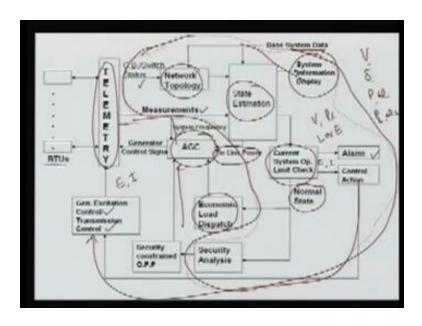
Here this is block diagram of the various functions of modern energy management systems. First, we will see here we start with the RTUs. RTUs are nothing but the remote terminal units by which we measure the power system data from the field and this data; it means this RTU gives information to this various modules and through the telemetry. So, this is the telemetry, and the RTUs are the large number in the power system; they are spread all over the world.
